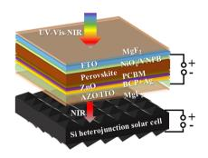
Designed multi-layer buffer for high-performance semitransparent wide-bandgap perovskite solar cells
