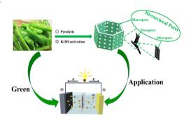
Green pepper-derived hierarchical porous carbon for supercapacitors with high performance
