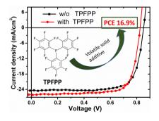
A fluorine functionalised phosphine based solid additive for morphology control and achieving efficient organic solar cells
