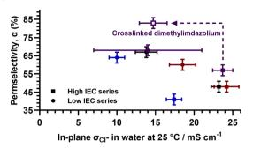
Changes in permselectivity of radiation-grafted anion-exchange membranes with different cationic headgroup chemistries are primarily due to water content differences
