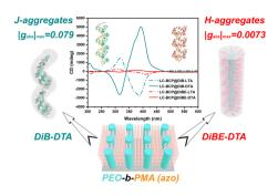
Chiral amplification induced by self-assembly of different aggregation states in liquid crystal block copolymer films with chiral response
