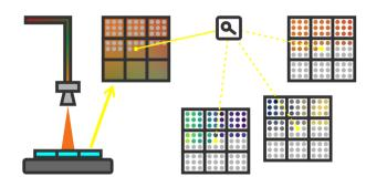
Accelerated screening of Cu-Ga-Fe oxide semiconductors by combinatorial spray deposition and high-throughput analysis
