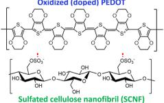
In situ polymerized PEDOT dispersions with sulfated cellulose nanofibrils for 1D and 2D conductors
