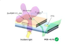
Aza-benzannulated-perylenebisimide-porphyrin dyad as an intensely absorbing donor in bulk-heterojunction organic solar cells
