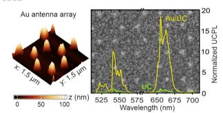
Enhancement of upconversion photoluminescence in phosphor nanoparticle thin films using metallic nanoantennas fabricated by colloidal lithography
