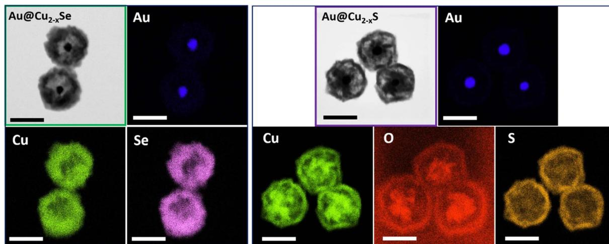
Fig. 4 Elemental distributions of Au, Cu, and Se in hollow dual-plasmonic Au@Cu<sub>2-x</sub>Se (left panel). Mapping images of Au, Cu, O, and S in hollow dual-plasmonic Au@Cu<sub>2-x</sub>S (right panel). Scale bar: 200 nm.
