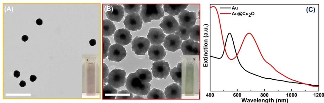
Fig. 1 Formation of the sacrificial hard templates. TEM images of (A) Au quasi-spherical nanoparticles and (B) Au@Cu<sub>2</sub>O core-shell NPs. Insets: color pictures of corresponding colloidal solutions of Au quasi-spherical NPs and Au@Cu<sub>2</sub>O core-shell NPs. Scale bars correspond to 200 nm. (C) The extinction spectra of colloidal Au and Au@Cu<sub>2</sub>O NPs (cuvette path length is 0.5 cm).
