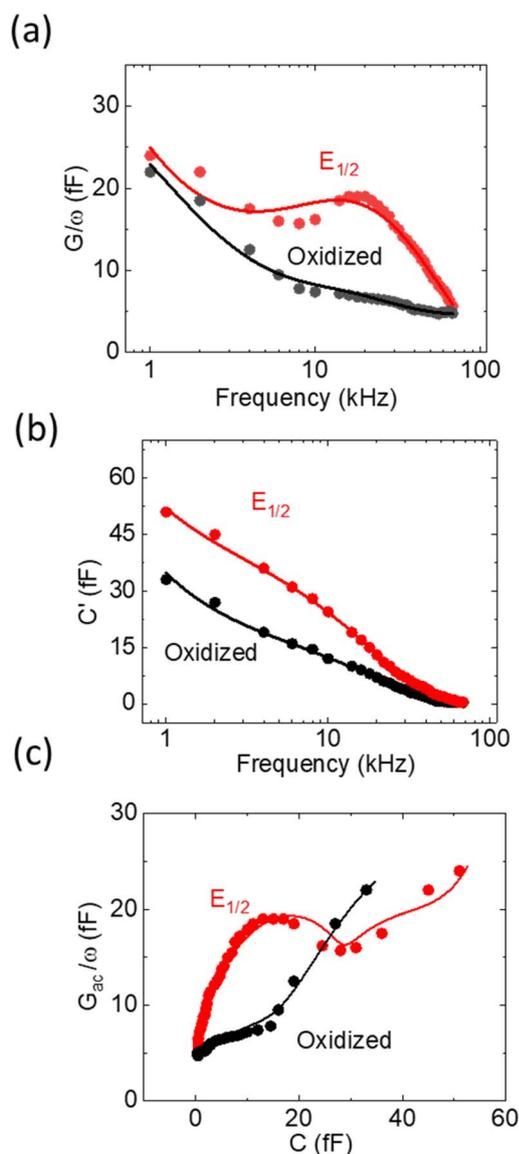
Fig. 4 Experimental results DLEIS, fitted to the analytical simulation (a) and (b) are Bode plots of  $C_{ac}$  and  $G_{ac}/\omega$ , the real and imaginary part of  $dQ/dV$ , respectively. The red circles and lines are the measured LEIS at  $E_{1/2}$  and the simulated data, respectively. The black circles and lines are measured LEIS at the oxidation potential and the simulated data. (c) is the Nyquist plot of (a) and (b).
