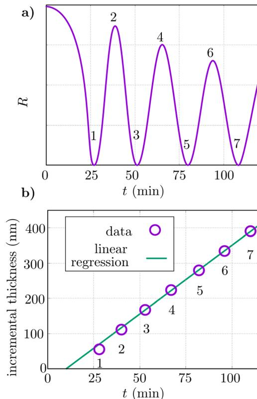
**Fig. 9** Schematic reflectance to depict the method to estimate the incubation period. (a) Typical reflectance  $R$  curve obtained during diamond deposition on seeded substrates as a function of time  $t$  where extrema are numbered. (b) Incremental thickness  $h$  as a function of  $t$  for the curve in (a). The values of  $h$  are calculated with (17).
