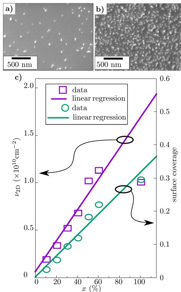
Fig. 4 Seed density. (a) SEM image of a sample seeded using a suspension of concentration  $x = 10\%$ . (b) SEM image of a sample seeded with an  $x = 100\%$  suspension. (c) Seed density  $\nu_{2D}$  and surface coverage as function of  $x$ . Density  $\nu_{2D}$  is defined as the number of isolated diamond particles in the image, divided by the total area. For the linear regression the value of  $\nu_{2D}$  for  $x = 100\%$  is not considered.
