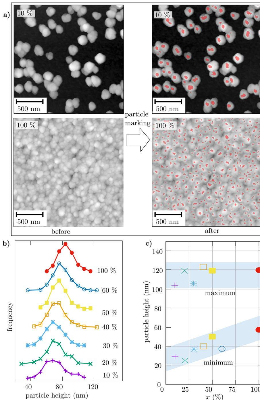
Fig. 7 AFM particle analysis. (a) AFM images of samples seeded with suspensions of concentration  $x = 10\%$  and  $x = 100\%$ , before and after applying the watershed method for marking particles. (b) Height distribution and (c) the maximum and the minimum height of particles found in the analysis of two AFM images of each sample.
