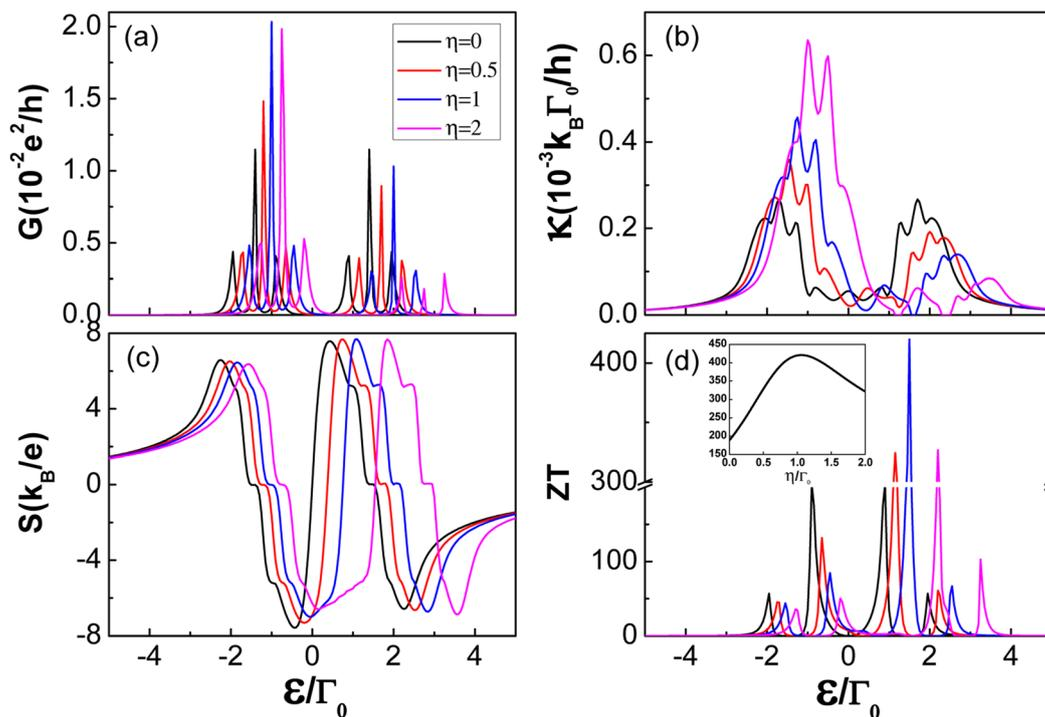
Fig. 8 (a) Electrical conductance  $G$ , (b) thermal conductance  $\kappa$ , (c) thermopower  $S$ , and (d) the figure of merit  $ZT$  as a function of asymmetry parameter  $\eta$ . Other parameters are the same as in Fig. 3.
