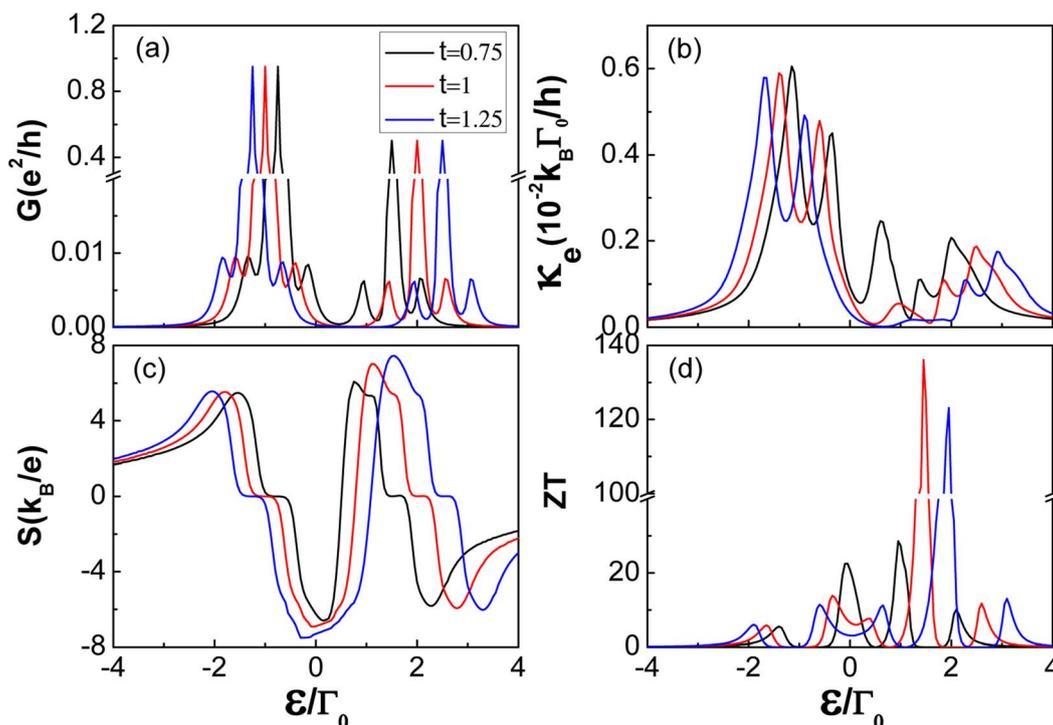
Fig. 5 Transport and thermoelectric coefficients: (a) electrical conductance  $G$ , (b) thermal conductance  $\kappa$ , (c) thermopower  $S$ , and (d) figure of merit  $ZT$  as a function of the dot energy level  $\varepsilon/\Gamma_0$ , under the indicated values of interdot coupling  $t$  for  $\Delta = 0.5$  and  $\eta = 1$  in the N-TTQD-S system. Other parameters are the same as in Fig. 3.
