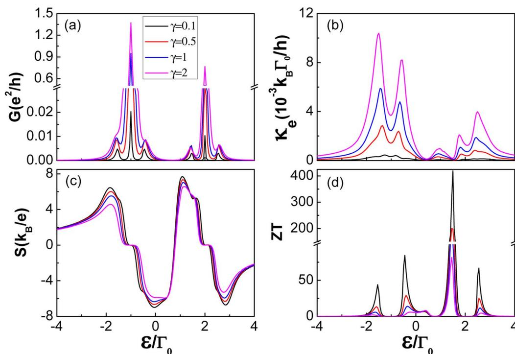
Fig. 7 Transport and thermoelectric coefficients: (a) electrical conductance  $G$ , (b) thermal conductance  $\kappa$ , (c) thermopower  $S$ , and (d) figure of merit  $ZT$ , as a function of the dot energy level  $\varepsilon/\Gamma_0$  under the indicated values of the asymmetry parameter  $\gamma(\Gamma_S/\Gamma_N)$  for  $\Delta = 0.5$ ,  $t = 1$  and  $\eta = 1$  in the TTQD device. Other parameters are the same as in Fig. 3.
