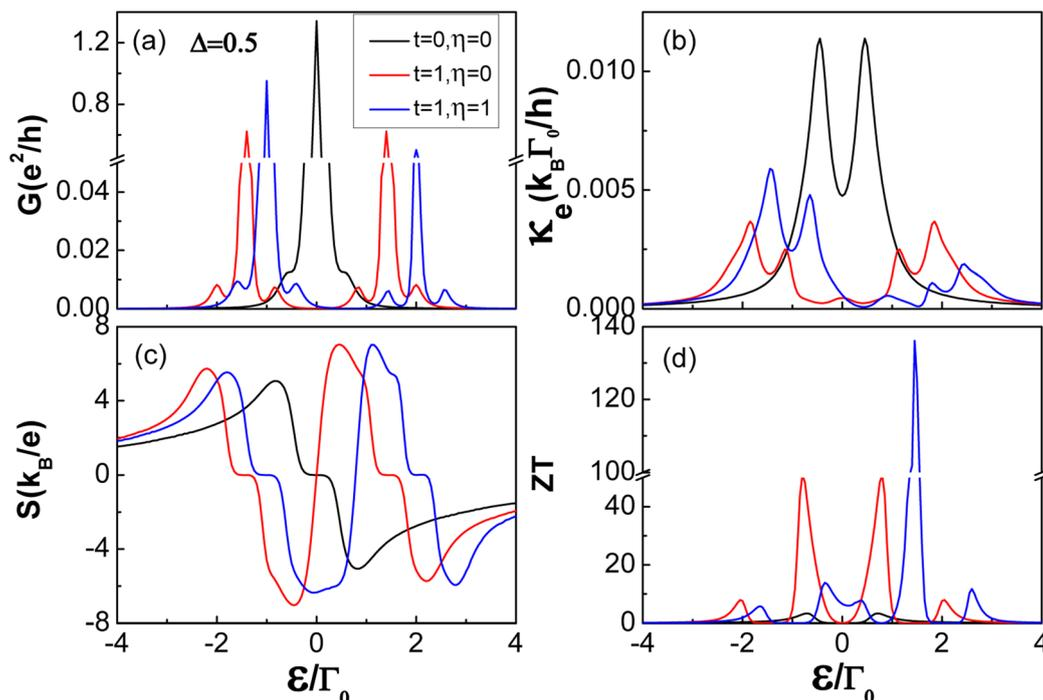
Fig. 3 Transport and thermoelectric coefficients: (a) electrical conductance  $G$ , (b) thermal conductance  $\kappa$ , (c) thermopower  $S$ , and (d) figure of merit  $ZT$  as a function of the quantum dot energy level  $\varepsilon/\Gamma_0$  in N-QD-S, N-TQD-S and N-TTQD-S – the three different systems for  $\Delta = 0.5$ . The other parameters are set as in Fig. 2.
