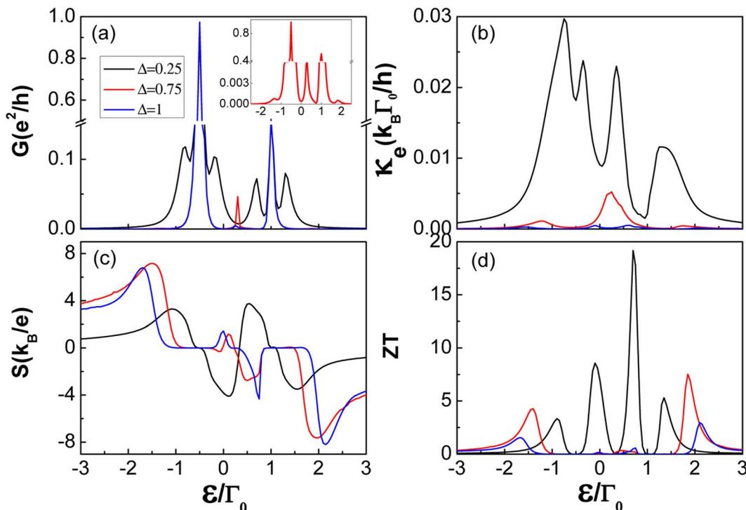
Fig. 4 Transport and thermoelectric coefficients: (a) electrical conductance  $G$ , (b) thermal conductance  $\kappa$ , (c) thermopower  $S$ , and (d) figure of merit  $ZT$  as a function of the dot energy level  $\varepsilon/\Gamma_0$ , under indicated values of superconducting gap  $\Delta$  for  $t = 0.5$  and  $\eta = 1$  in the N-TTQD-S system. Other parameters are the same as in Fig. 3.
