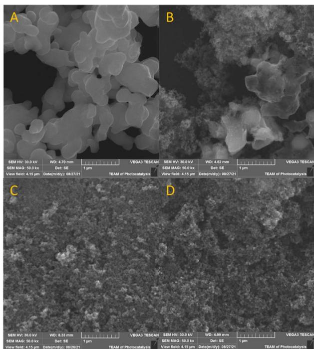
Fig. 4 SEM images of bare Ag<sub>2</sub>O (a), TiO<sub>2</sub>/Ag<sub>2</sub>O (b), TiO<sub>2</sub>/Ag<sub>2</sub>O<sub>hν</sub>30s (c), and TiO<sub>2</sub>/Ag<sub>2</sub>O<sub>hν</sub>2h (d).
