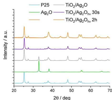
Fig. 1 X-ray diffractograms of the TiO<sub>2</sub>/Ag<sub>2</sub>O composite: as-prepared and modified under irradiation. Raw components (P25 and as-synthesized Ag<sub>2</sub>O) are shown for reference.
