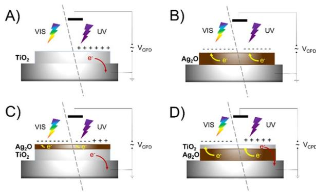
**Scheme 1** Visualization of photogenerated charge transfer in SPV measurements for  $\text{TiO}_2$  (a),  $\text{Ag}_2\text{O}$  (b),  $\text{Ag}_2\text{O}$  on the top of  $\text{TiO}_2$  (c) and  $\text{TiO}_2$  on the top of  $\text{Ag}_2\text{O}$  (d).
