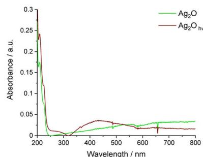
Fig. 7 UV-vis absorption spectra of bare Ag<sub>2</sub>O before and after irradiation (2 h).
