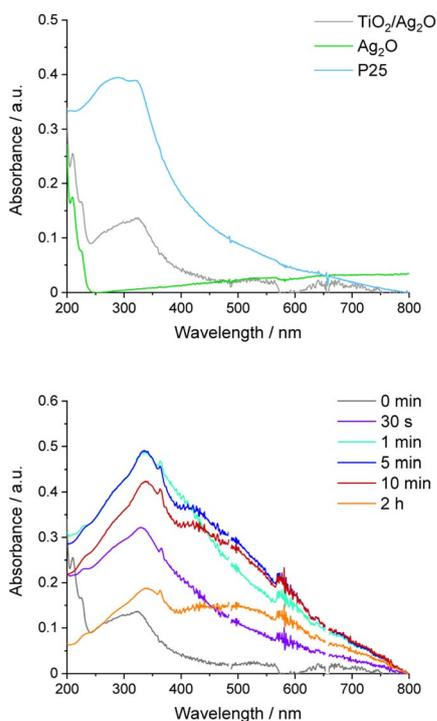
Fig. 8 UV-vis spectra of the TiO<sub>2</sub>/Ag<sub>2</sub>O composite and its components (upper picture); UV-vis spectra recorded at decisive time intervals of TiO<sub>2</sub>/Ag<sub>2</sub>O irradiation (lower picture).
