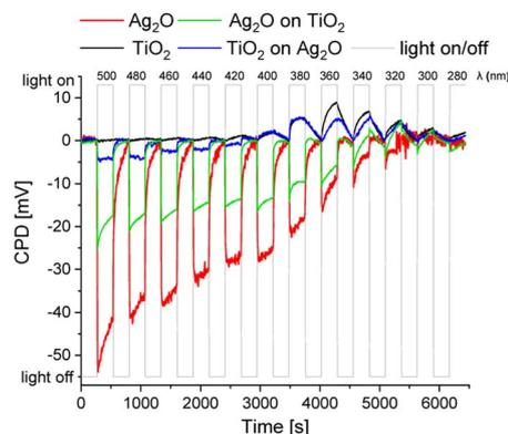
Fig. 10 SPV for TiO<sub>2</sub>, Ag<sub>2</sub>O and layered systems: TiO<sub>2</sub> on top of Ag<sub>2</sub>O and vice versa.
