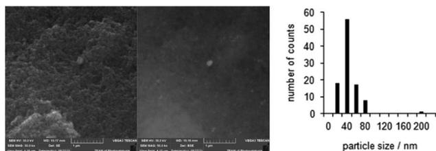
Fig. 5 SEM image of the selected area of the TiO<sub>2</sub>/Ag<sub>2</sub>O<sub>hν</sub>2h composite recorded with SE (left) and BSE (middle) detectors along with the particle size distribution (right).
