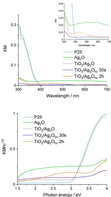
Fig. 6 DRS spectra of examined materials: Kubelka–Munk function (upper picture) and Tauc transformation (lower picture). The inset shows the magnification in the range of the SPR band of silver nanoparticles.
