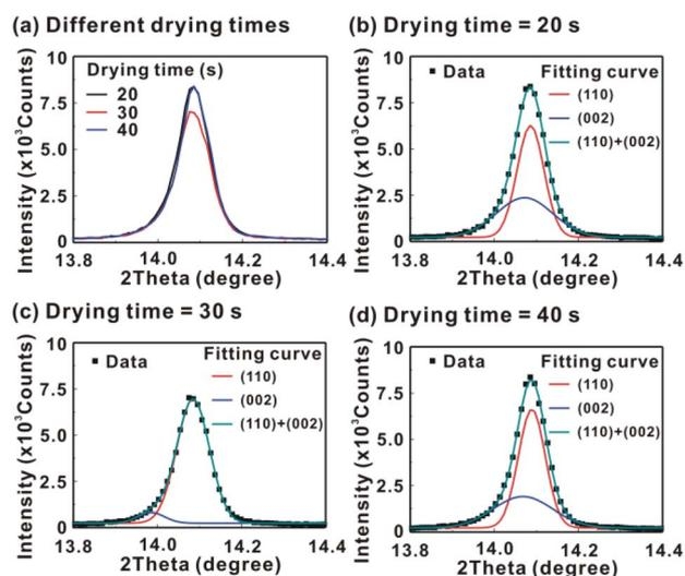
Fig. 6 (a) Main X-ray diffraction patterns of the MAPbI<sub>3</sub>/P3CT-Na/ITO/glass samples fabricated with different drying times (DTs). (b) Fitting curves, DT = 20 s; (c) fitting curves, DT = 30 s; (d) fitting curves, DT = 40 s.
