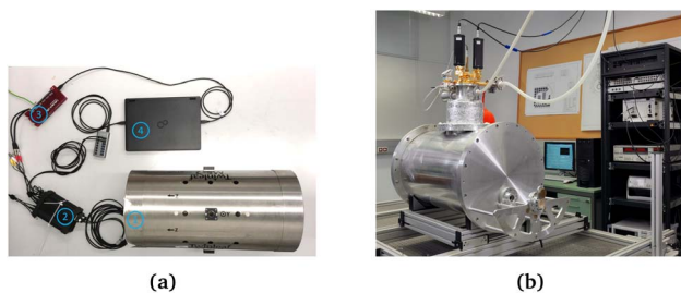
Fig. 3 (a) Tabletop TNM setup based on OPMs. The sample is placed inside the Twingleaf MS-2 shield (1) together with the two QZFM. QZFM electronics (2) control the sensors and a laptop (4) serves for driving the DAQ Labjack U6 (3) in stream mode, running the QZFM electronics and collecting the data. The sample is at an average distance of 13.5 mm from the gas cell with the polarized Rb atoms. (b) In-house developed SQUID setup for reference measurements. A superconducting Nb magnetic shield and 6 SQUID sensors are kept at LHe temperature; the sample is placed in a bore through the setup and kept at an average temperature of 43.0 \pm 0.5 °C to match the sample temperature in the tabletop setup. An average distance of 23.5 mm is measured between the pickup coils of the SQUID sensors and the sample. Only one sensor is used for the TNM measurement.
