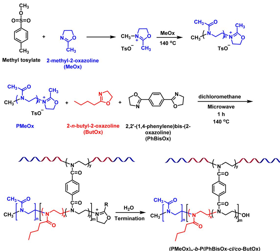
Scheme 1 Synthetic route to prepare CCS (PMeOx)<sub>n</sub>-b-P(PhBisOx-*cl/co*-ButOx) by microwave-assisted CROP.
