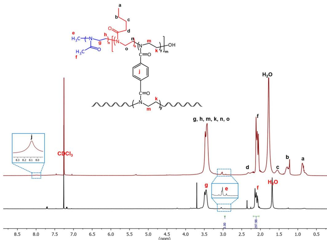
**Fig. 1** <sup>1</sup>H NMR of the PMeOx arm (black) and (PMeOx)<sub>59</sub>-*b*-P(PhBisOx-*cl*/*co*-ButOx) (red) (500 MHz, CDCl<sub>3</sub>, 25 °C).
