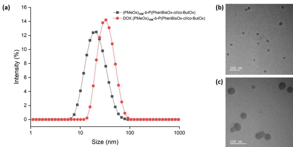
Fig. 3 (a) DLS traces of (PMeOx)<sub>106</sub>-b-P(PhBisOx-cl/co-ButOx) (black) (concentration: 2 mg mL<sup>-1</sup>) and DOX-loaded (PMeOx)<sub>106</sub>-b-P(PhBisOx-cl/co-ButOx) (red) (concentration: 1 mg mL<sup>-1</sup>) and TEM images of (b) (PMeOx)<sub>106</sub>-b-P(PhBisOx-cl/co-ButOx) and (c) DOX-loaded (PMeOx)<sub>106</sub>-b-P(PhBisOx-cl/co-ButOx).
