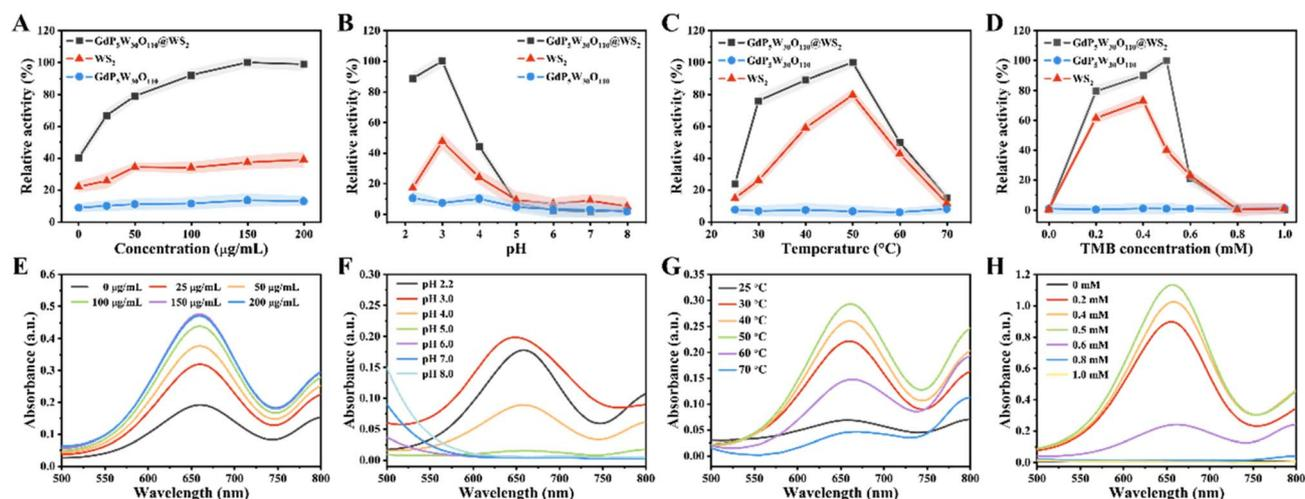
Fig. 3 The optimization of (A) concentration, (B) pH, (C) temperature and (D) TMB concentration for the peroxidase-like activity of  $\text{GdP}_5\text{W}_{30}\text{O}_{110}@WS_2$ ,  $\text{GdP}_5\text{W}_{30}\text{O}_{110}$  and  $WS_2$  calculated from the corresponding absorbance values (E–H). The maximum point in every curve was set as 100%. Error bars represent the standard error derived from three independent measurements.
