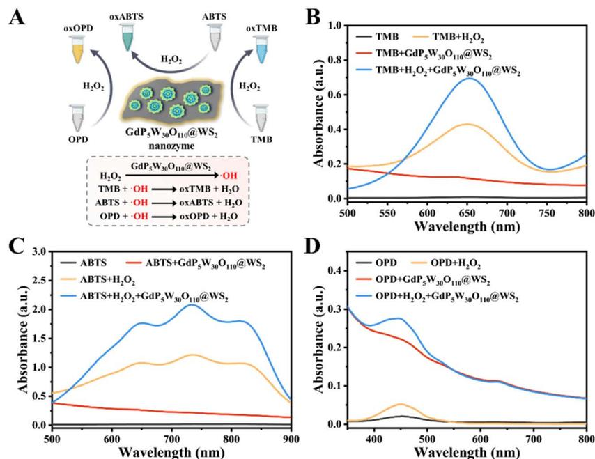
Fig. 2 (A) Schematic illustration of the mechanism for the peroxidase-like activity evaluation of  $\text{GdP}_5\text{W}_{30}\text{O}_{110}@WS_2$  applying TMB, OPD and ABTS as substrates. UV-vis-NIR adsorption spectra of the catalyzed oxidation of (B) TMB, (C) ABTS and (D) OPD after 15 min of incubation with PBS,  $\text{GdP}_5\text{W}_{30}\text{O}_{110}@WS_2$ ,  $\text{H}_2\text{O}_2$  and  $\text{H}_2\text{O}_2 + \text{GdP}_5\text{W}_{30}\text{O}_{110}@WS_2$  at pH 4.0.
