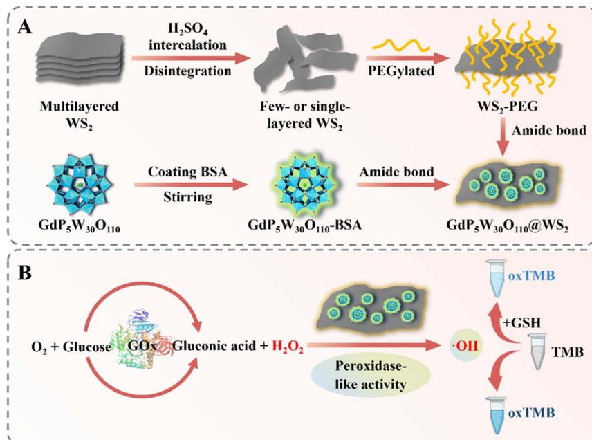
**Scheme 1** (A) Schematic illustration of the general synthetic procedures of the  $GdP_5W_{30}O_{110}@WS_2$  nanozymes; (B) Mechanism description of  $GdP_5W_{30}O_{110}@WS_2$  nanozymes with peroxidase-like activity for the colorimetric detection of biomolecules, including  $H_2O_2$ , GSH and glucose.
