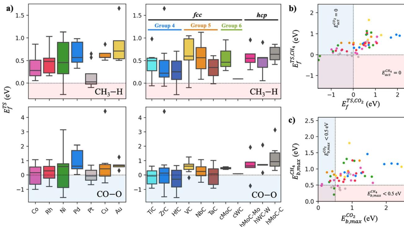
Fig. 5 (a) Distribution of  $E_f^{TS}$  for  $CH_4$  (top) and  $CO_2$  (bottom) dissociation for each metal (left) and TMC support (right). (b) Scatter plot of  $E_f^{TS}$  for  $CH_4$  dissociation against  $E_f^{TS}$  for  $CO_2$  dissociation. (c) Scatter plot of  $E_{b,max}$  for  $CH_4$  dissociation against  $E_{b,max}$  for  $CO_2$  dissociation.
