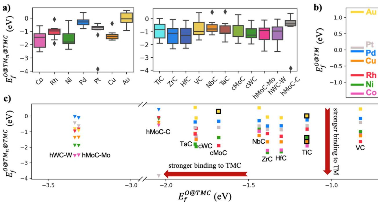
Fig. 4 (a) Distribution of  $E_{\text{f}}^{\text{O@TM}_n\text{@TMC}}$  for each metal (left) and TMC support (right). (b) Calculated values of  $E_{\text{f}}^{\text{O@TM}}$ . (c) Scatter plot of  $E_{\text{f}}^{\text{O@TM}_n\text{@TMC}}$  against  $E_{\text{f}}^{\text{O@TMC}}$ . The four squares with a black outline correspond to TM<sub>n</sub>@TMC systems that have been reported experimentally to be stable for various reactions of industrial importance.
