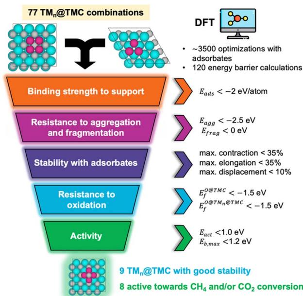
Fig. 6 High-throughput screening workflow developed to identify promising  $TM_n@TMC$ s catalysts for  $CH_4$  and  $CO_2$  conversion. Cyan and grey spheres represent metal and C atoms from the TMC, respectively, while magenta spheres represent the supported cluster.
