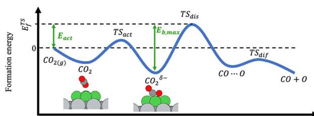
Fig. 1 Example of the reaction profile of  $\text{CO}_2$  adsorption and dissociation on a supported cluster.  $\text{TS}_{\text{act}}$ ,  $\text{TS}_{\text{dis}}$  and  $\text{TS}_{\text{dif}}$  are the TSs for the activation, dissociation, and diffusion steps, respectively. Light grey and green spheres represent the metal atoms from the carbide and the supported cluster, respectively, and dark grey and red spheres represent carbon atoms and oxygen atoms, respectively.
