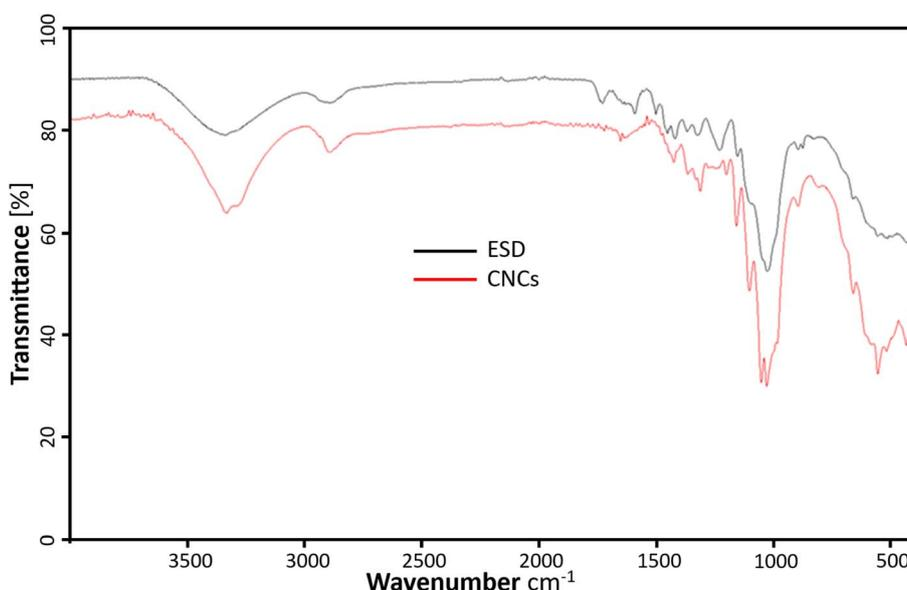
Fig. 5 ATR-FTIR profiles showing the chemical composition of cellulose nanocrystals (red), and Eucalyptus grandis saw dust (black).
