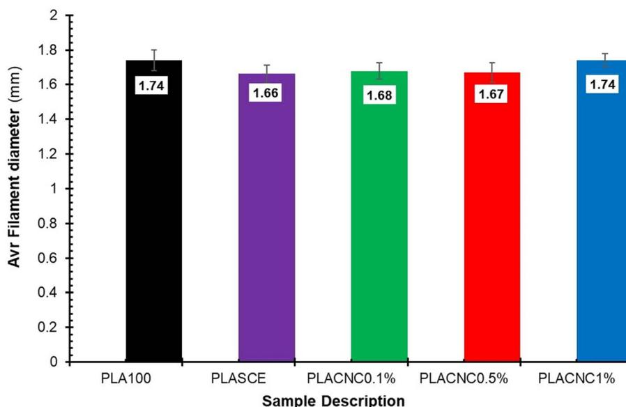
Fig. 15 The average filament diameters of the PLA and PLA/CNC bionanocomposites filaments.
