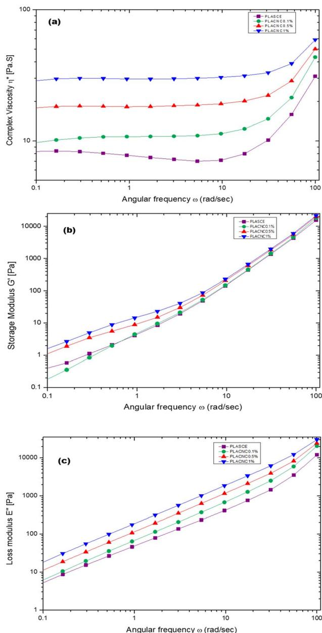
Fig. 17 Melt rheological behaviour of PLA/CNC bionanocomposites showing the evolution of; (a) complex viscosity ( $\eta^*$ ), (b) storage ( $G'$ ) modulus, (c) loss ( $G''$ ) modulus.
