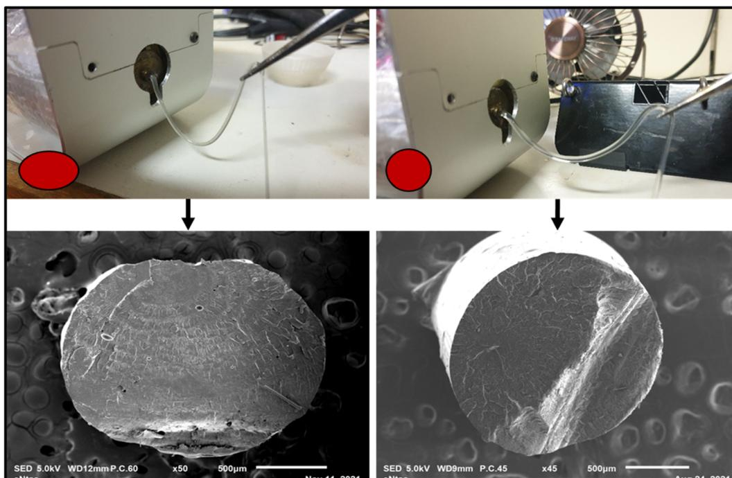
Fig. 13 Enhanced melt strength during filament extrusion: minimal drooping of filament during extrusion.
