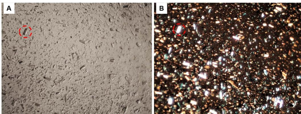
Fig. 4 Optical microscopy image of re-dispersed cellulose nanocrystals (CNCs); (A), high contrast image under normal light, (B) CNCs showing birefringence under polarised light (64 $\times$  magnification).
