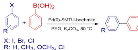
Scheme 2 Suzuki–Miyaura coupling reaction of aryl halides and phenylboronic acid catalyzed by Pd(0)-SMTU-boehmite.
