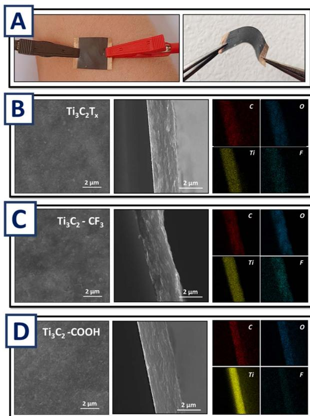
Fig. 2 (A) Photos of created humidity sensors based on pristine or grafted  $Ti_3C_2T_x$  flakes deposited on flexible PP membrane; (B)–(D) SEM images and corresponded EDX mapping of thin films created from pristine  $Ti_3C_2T_x$  flakes and flakes grafted with  $-C_6H_4-COOH$  and  $-C_6H_4-CF_3$  flakes.
