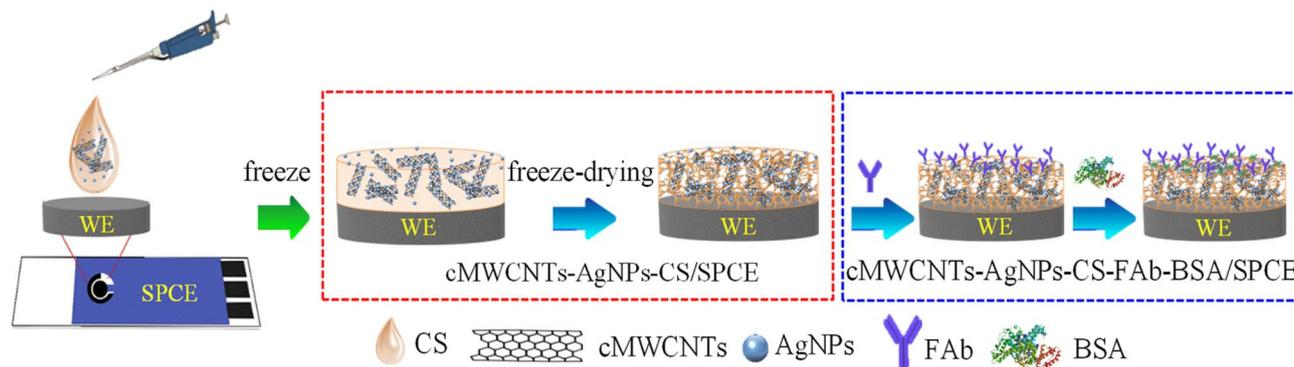
Fig. 1 Schematic illustration of the preparation of cMWCNTs-AgNPs-CS-Fab-BSA/SPCE.
