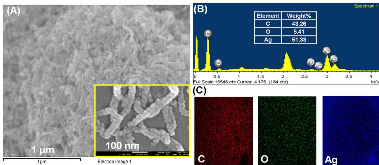
Fig. 5 (A) The SEM images of the cMWCNTs-AgNPs (inset: 2 000 00 $\times$  magnification). (B) The EDS spectrum of cMWCNTs-AgNPs. (C) The EDS mapping of C, O and Ag elements in cMWCNTs-AgNPs.
