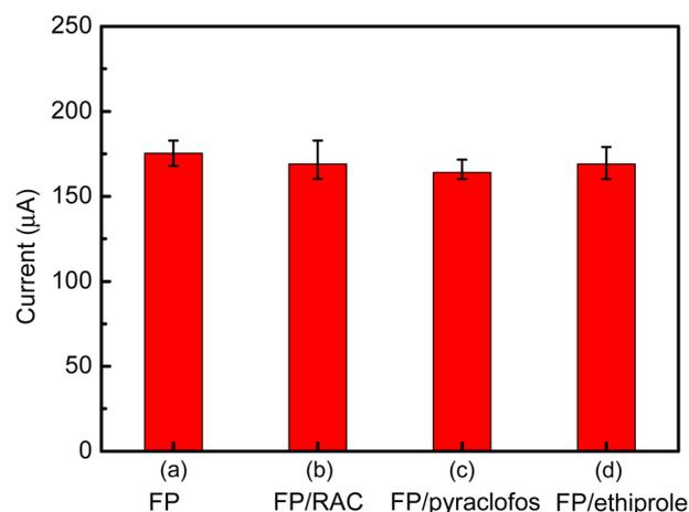
Fig. 14 Selectivity of the immunosensor. The anodic peak currents of the immunosensor in the presence of 1 ng per mL FP and various interfering substances (10 ng mL<sup>-1</sup>) in a 0.1 M PBS solution (pH 7.5) containing 10 mM [Fe(CN)<sub>6</sub>]<sup>3-/4-</sup>: (a) 1 ng per mL FP; (b) 1 ng per mL FP + 10 ng per mL RAC; (c) 1 ng per mL FP + 10 ng per mL pyraclofos, and (d) 1 ng per mL RAC + 10 ng per mL ethiprole.
