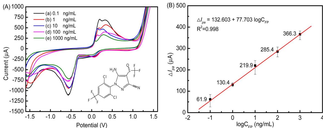
Fig. 12 (A) The CV responses of the cMWCNTs-AgNPs-CS-Fab-BSA/SPCE immunosensor in 0.1 M PBS (pH 7.5) containing various concentrations of FP (a–e: 0.1, 1, 10, 100 and 1000  $\text{ng mL}^{-1}$ ) (inset: the chemical structure of FP). (B) The calibration curve of current change ( $\Delta I_{\text{pa}}$ ) against log FP concentration.
