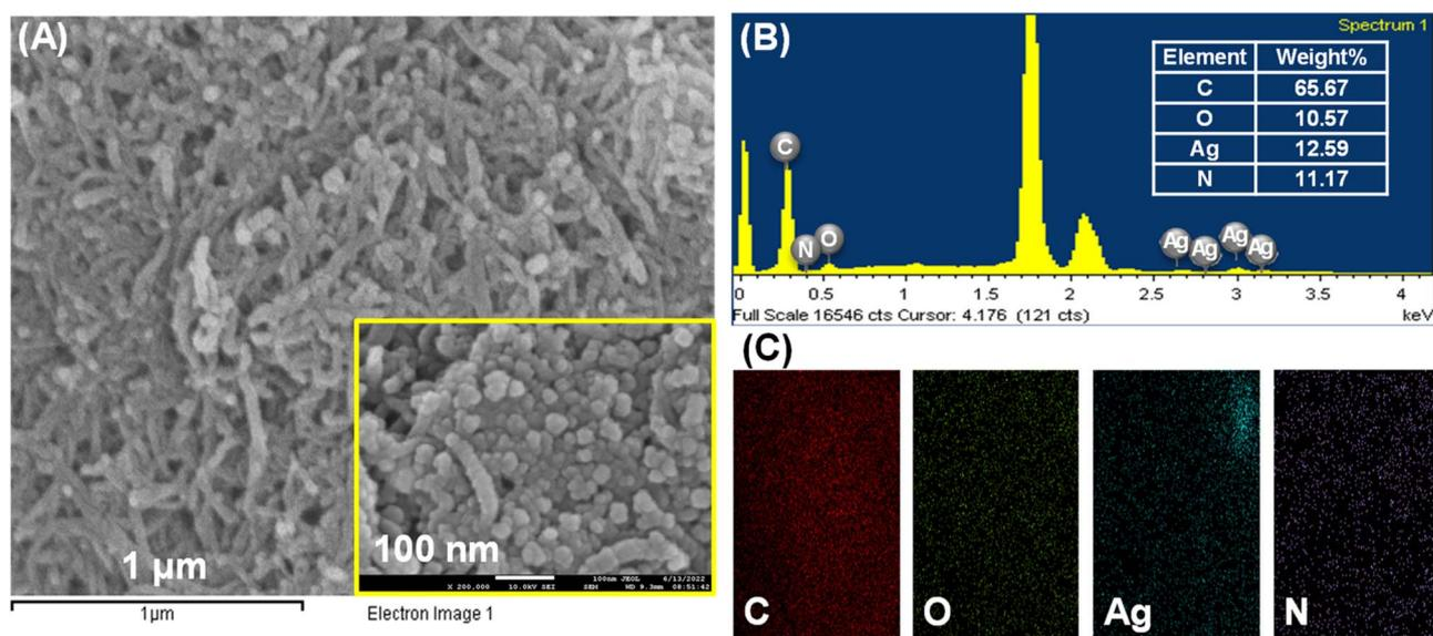
Fig. 6 (A) The SEM images of the cMWCNTs-AgNPs-CS composite (inset: 2 000 00 $\times$  magnification). (B) The EDS spectrum of cMWCNTs-AgNPs-CS. (C) The EDS mapping of C, O, Ag, and N elements in cMWCNTs-AgNPs-CS.
