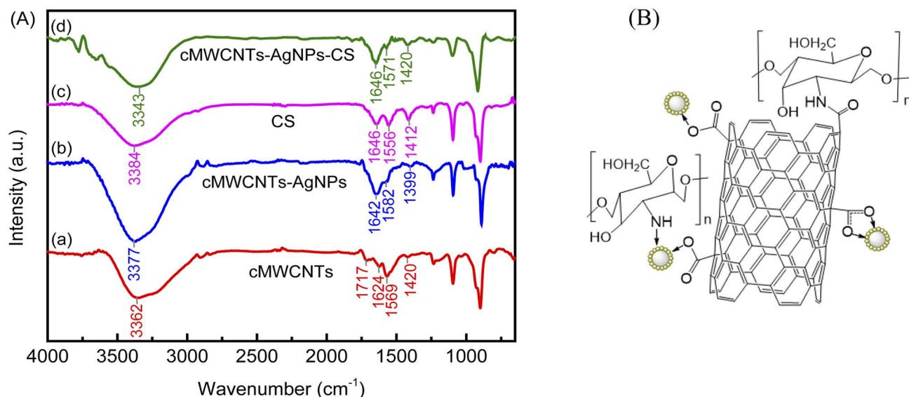
Fig. 3 (A) The FTIR spectra and (B) structure of the cMWCNTs-AgNPs-CS composite.
