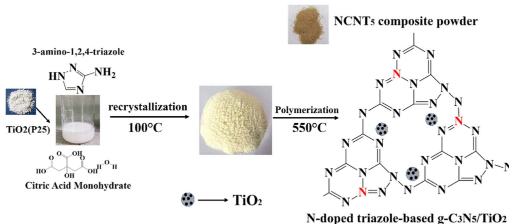
Scheme 1 The construction of the NCNT x S-scheme heterojunction photocatalyst.
