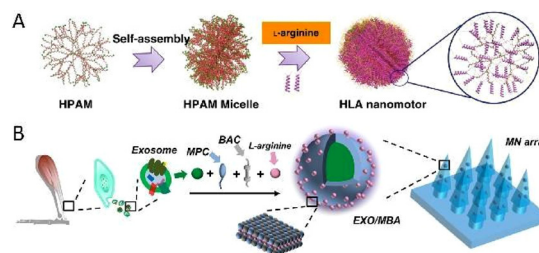
Fig. 3 (A) Fabrication process of the NO-driven nanomotor composed of HPAM and L-arginine. This figure has been reproduced from ref. 49 with permission from the Springer Nature, copyright 2019. (B) Manufacturing procedure of exosome-loaded microneedle arrays modified by NO-driven nanomotors. This figure has been adapted from ref. 50 with permission from the American Chemical Society, copyright 2021.
