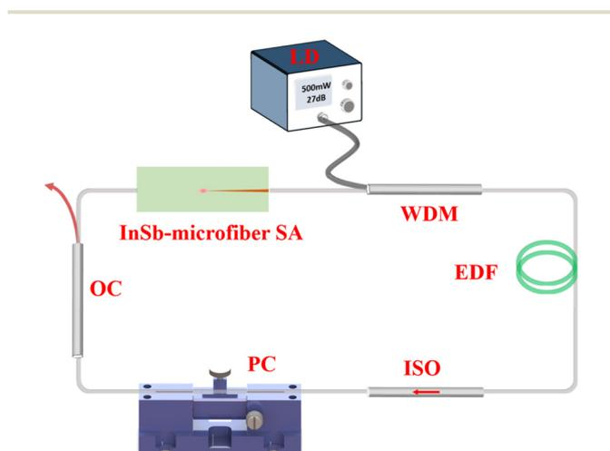
Fig. 7 The setup of a mode-locked EDF laser.
