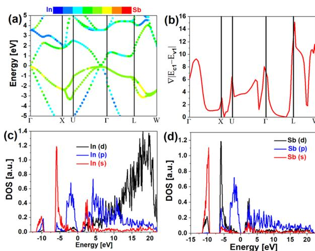
Fig. 2 (a) Band structure of bulk InSb; (b) modulus of a gradient of difference for bulk InSb; (c) DOS of In atoms; and (d) DOS of Sb atoms.
