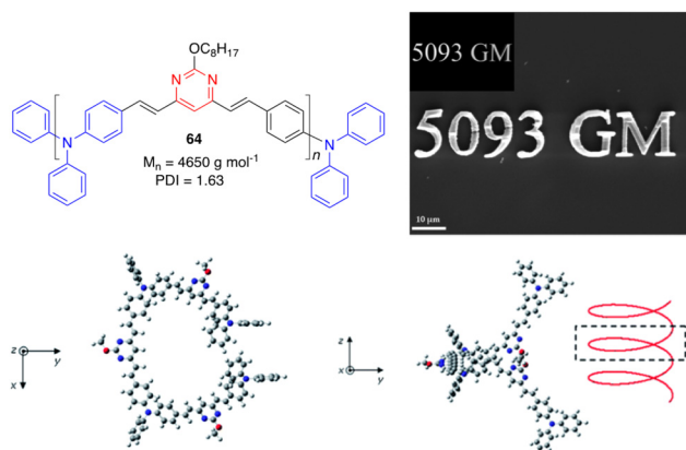
Fig. 27 Top left: Structure of the oligomer 64 . Top right: SEM image of a \mu -structure fabricated upon excitation at 800 nm of a diacrylate resin with 64 as the TPA sensitizer. Inset: 2D model master. Bottom: Optimized geometries of 64 associating three monomer units (PBE0/6-31G(d) level). Adapted with permission from ref. 26 (Copyright 2013, Royal Chemical Society).
