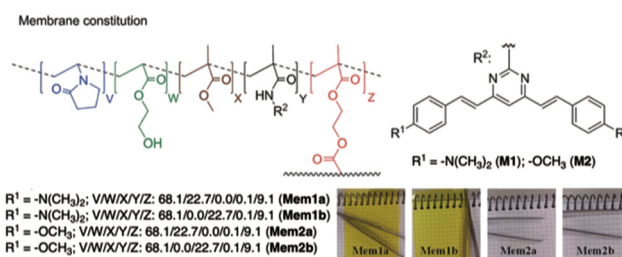
Fig. 11 Structure of the polymer membrane designed by Pablos and coworkers. Reproduced with permission from ref. 43 (copyright 2014, Royal Chemical Society).
