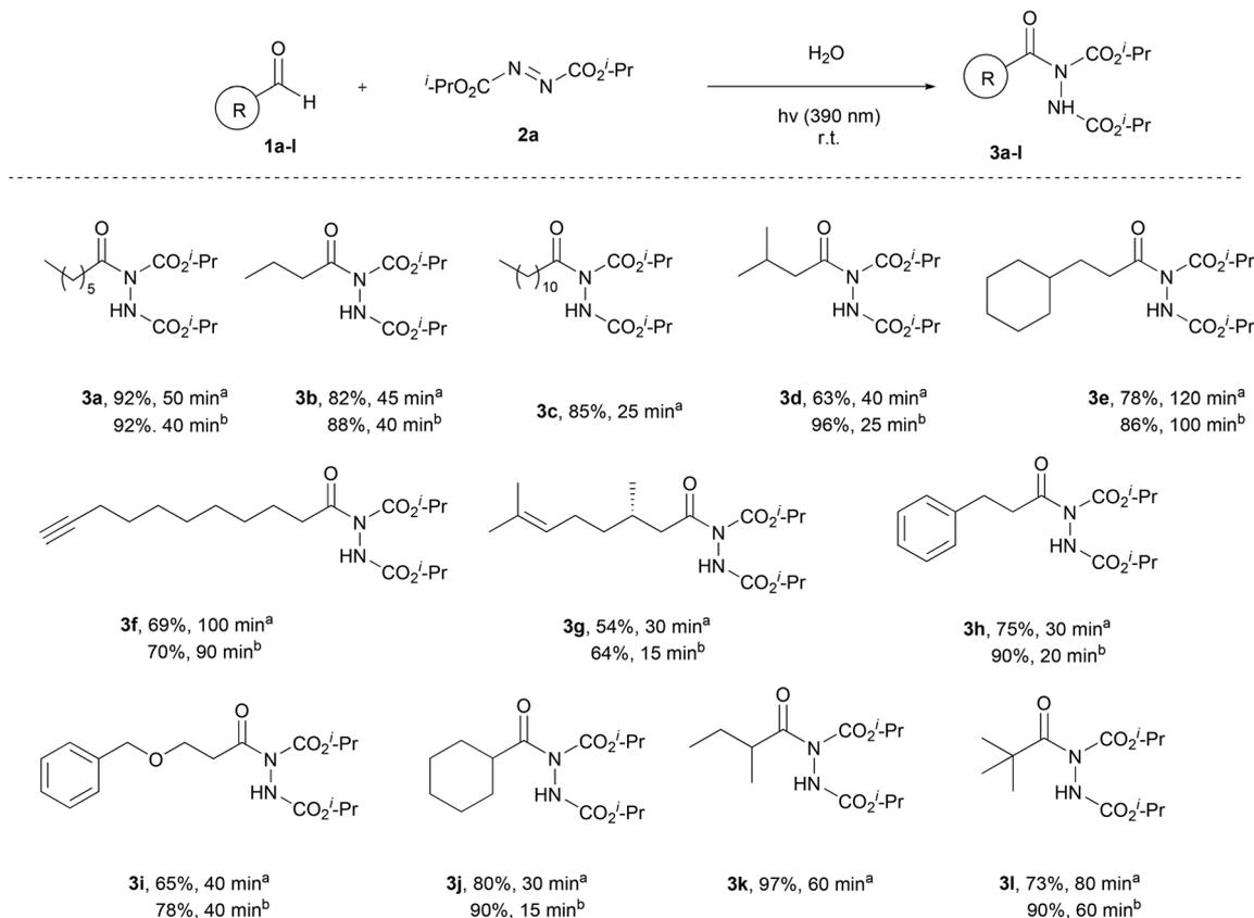
**Scheme 3** Substrate scope – aliphatic aldehydes. <sup>a</sup> Reaction time and yield of the isolated product, when 1.5 equiv. of aldehyde were used. <sup>b</sup> Reaction time and yield of the isolated product, when 2.0 equiv. of aldehyde were used.
