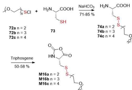
Fig. 45 Approach utilizing the equivalent of an “-S<sup>+</sup>” moiety for the synthesis of disulfide-containing monomers.
