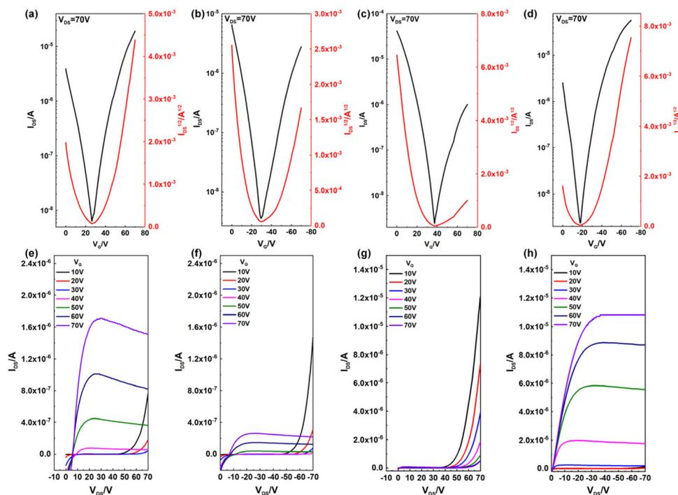
**Fig. 5** n-Type (a and c) transfer and (e and g) output characteristics of (a and e) PDPPMeBTzO and (c and g) PDPPMeBTz at 250 °C. p-Type (b and d) transfer and (f and h) output characteristics of (b and f) PDPPMeBTzO and (d and h) PDPPMeBTz at 250 °C.
