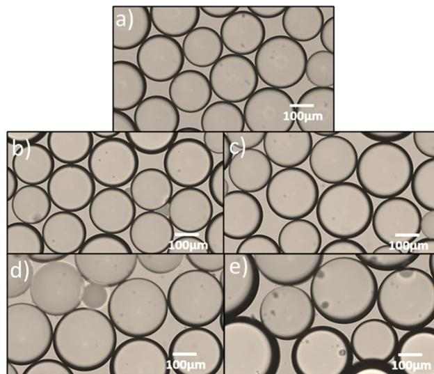
**Fig. 6** Optical micrographs of *n*-dodecane droplets stabilised with 0.1 wt% aqueous solutions of mixed LMw-PVA-88 to HMw-PVA-88 at the following volume ratios; (a) 9:1, (b) 7:3, (c) 1:1, (d) 3:7 and (e) 1:9. The images show changes in the droplet size and more importantly the droplet uniformity at the different polymer blend ratios. The stirred paddle rotational speed and the dispersed phase injection rate was kept constant at 1000 rpm and 0.1 mL min<sup>-1</sup> respectively.
