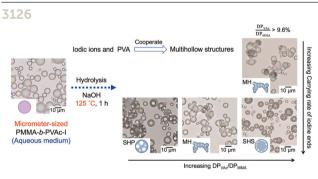
Iodine-influenced morphological evolution of micrometer-sized poly(methyl methacrylate)block-poly(vinyl acetate) particles upon hydrolysis
