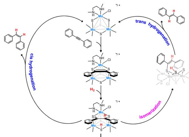
**Fig. 2** Simplified catalytic cycle for the semihydrogenation of dpa in the presence of Mo<sub>3</sub>S<sub>4</sub> clusters.
