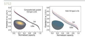
Boosting the voltage/capacity stability of O2-type Li-rich layered cathodes by tailoring transition metal distribution for Li-ion batteries
