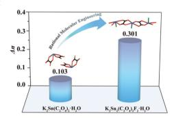
The transformation of a zero-dimensional cluster into a one-dimensional chain structure achieving a dramatically enhanced birefringence in tin(II)-based oxalates
