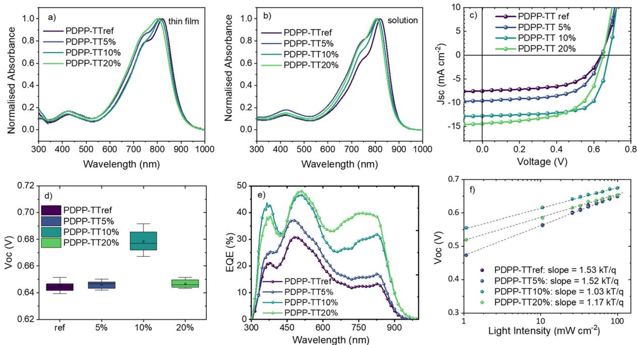
**Fig. 2** Normalized UV-Vis absorption spectra of different PDPP-TT polymer analogs in (a) thin films (spin-coated from 5 mg mL<sup>-1</sup> in CB) and (b) solutions (CB). (c) *J*-*V* characteristics, (d) box-plot depicting the statistical distribution of *V*<sub>oc</sub>, (e) EQE, and (f) intensity-dependent *V*<sub>oc</sub> measurements for OSCs with different PDPP-TT donor polymer analogs.
