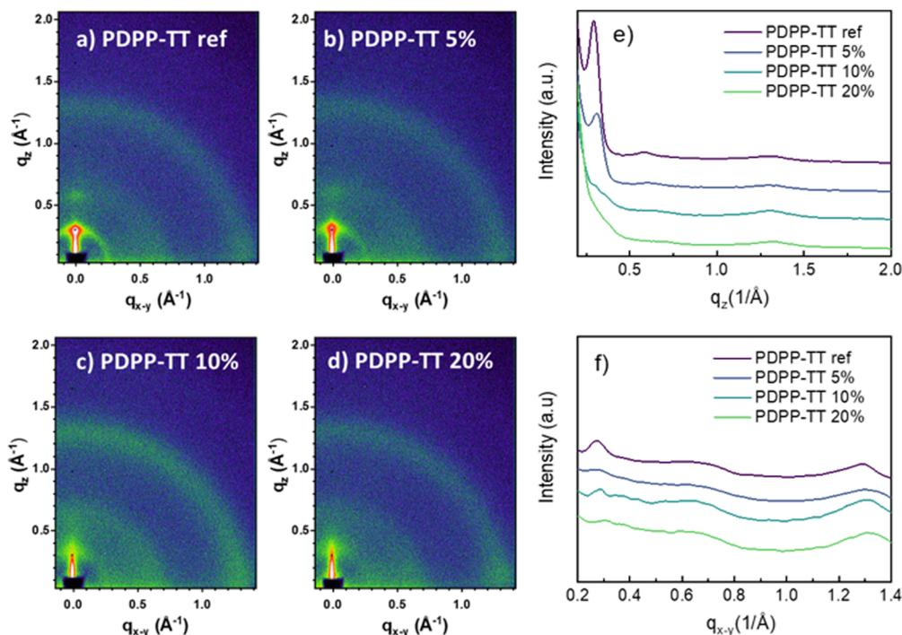
Fig. 5 2D-GIXRD profiles of polymer-PC<sub>71</sub>BM BHJ films with DPP polymer analogs (a) PDPP-TTref, (b) PDPP-TT5%, PDPP-TT10%, and PDPP-TT20%, (e) and (f) show the respective line-cuts.
