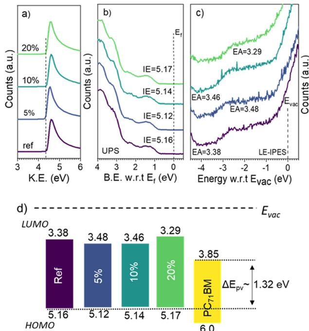
**Fig. 3** (a and b) Ultraviolet photoelectron spectroscopy (UPS), (c) low-energy inverse photoelectron spectroscopy (LE-IPES) spectra of PDPP-TT polymer analogs, and (d) schematic depicting the measured frontier molecular orbital energies of PDPP-TT polymer analogs and the resultant photovoltaic gap ( $\Delta E_{pv}$ ).
