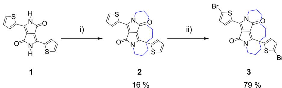
Scheme 1 Synthesis of encapsulated DPP monomer **3** (i) 1,10-dibromodecane, K<sub>2</sub>CO<sub>3</sub>, 18-crown-6, DMF, 120 °C, 18 h; (ii) NBS, CHCl<sub>3</sub>, 50 °C, 5 h.
