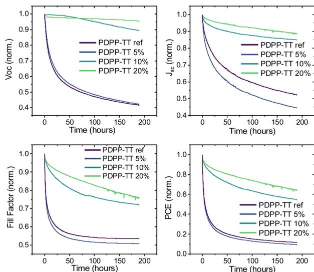
Fig. 6 Photostability of polymer-PC<sub>71</sub>BM BHJ OSCs incorporating different PDPP-TT polymer analogs with varying amounts of molecular encapsulation as donor material.
