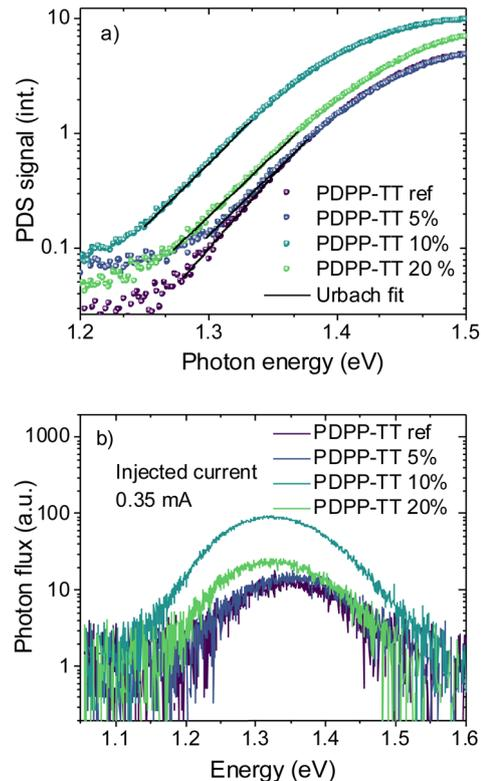
**Fig. 4** (a) Photothermal deflection spectroscopy (PDS) spectra of polymer-PC<sub>71</sub>BM BHJ blend films, (b) electroluminescence (EL) spectra (uncorrected for detector sensitivity) measured at the same exposure time, of OSCs based on BHJ blends having various PDPP-TT polymer analogs with varying amounts of encapsulated units in the polymer backbone.
