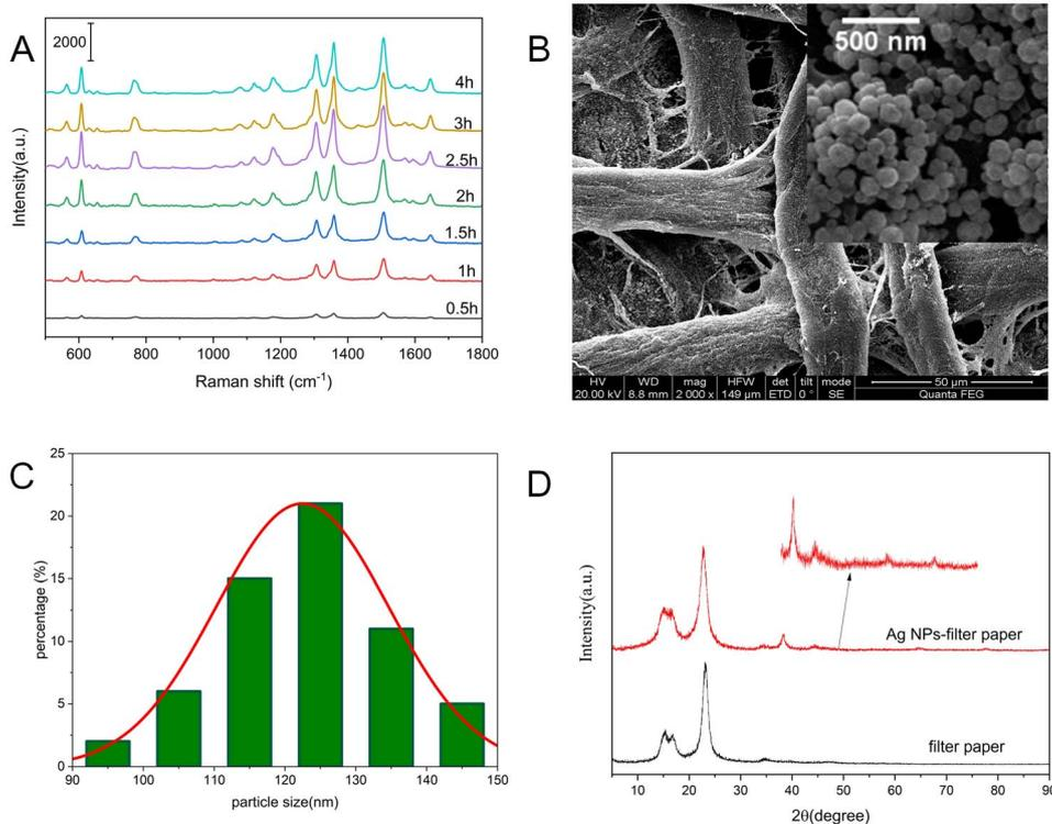
Fig. 2 (A) The SERS spectra of R6G ( $10^{-7}$  M) measured on Ag NPs-filter paper substrate with different silver mirror reaction time; (B) SEM image of the Ag NPs-filter paper substrate. Inset is the higher magnification image; (C) histograms of size distribution of Ag NPs on filter; (D) XRD spectra of filter paper and the Ag NPs-filter paper. Insets are the partial enlarged image.
