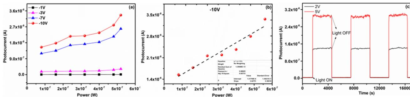
Fig. 6 Photoreponse performance of the COF366-QD device (a) upon irradiation with different power of 514 nm visible light and bias voltages in reverse bias Region, (b) at  $-10$  V (c) on/off switching of photocurrent at the bias voltage of 2 V and 5 V.
