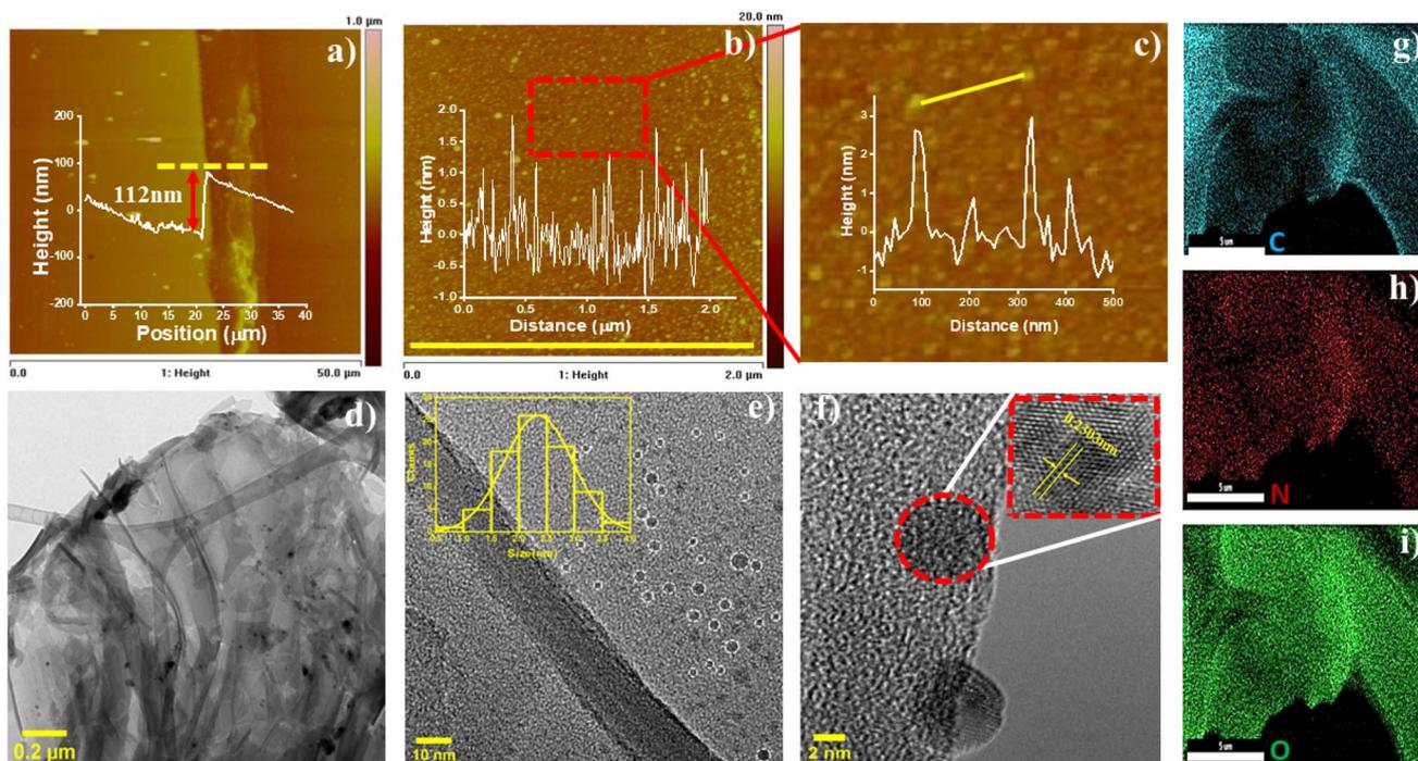
Fig. 4 (a–c) AFM images and (d–f) Transmission electron micrograph of the *in situ* CVD deposited COF366-QDs thin-film; inset (e): the particle size distribution histograms with Gaussian fitting where the marked black dots indicate the Quantum dots embedded in the COF layer; inset (f) HRTEM image of the COFQDs and (g–i) EDS elemental mapping of the COFQD thin-film.
