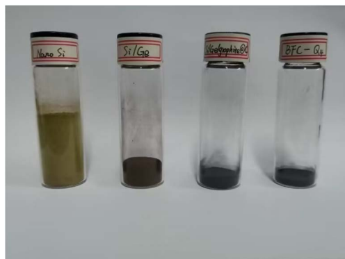
Fig. 3 Photographs of ball-milled Si (nano Si), Si/Ge, Si/Ge/graphite@C composite and artificial graphite (BFC-Q4).
