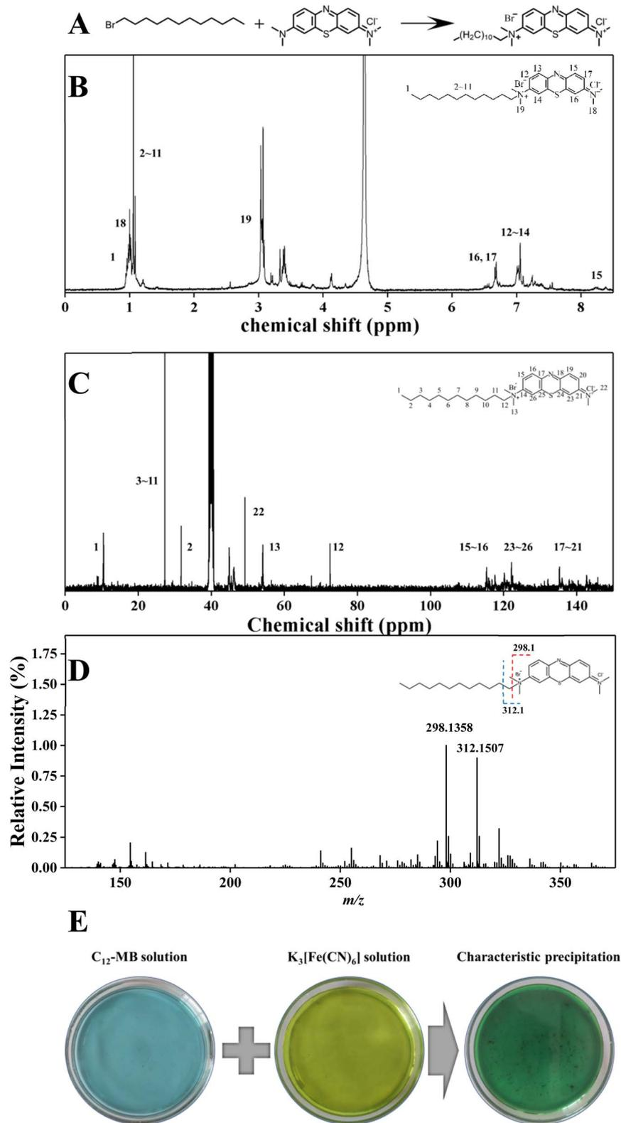
**Fig. 1** The synthesis and structural characterization of amphiphilic  $C_{12}$ -MB photosensitizers. (A) The synthesis diagram. (B)  $^1H$  NMR spectra. (C)  $^{13}C$  NMR spectra. (D) High resolution electrospray ionization mass spectra. (E) Identification of positive charge of quaternary ammonium salt.
