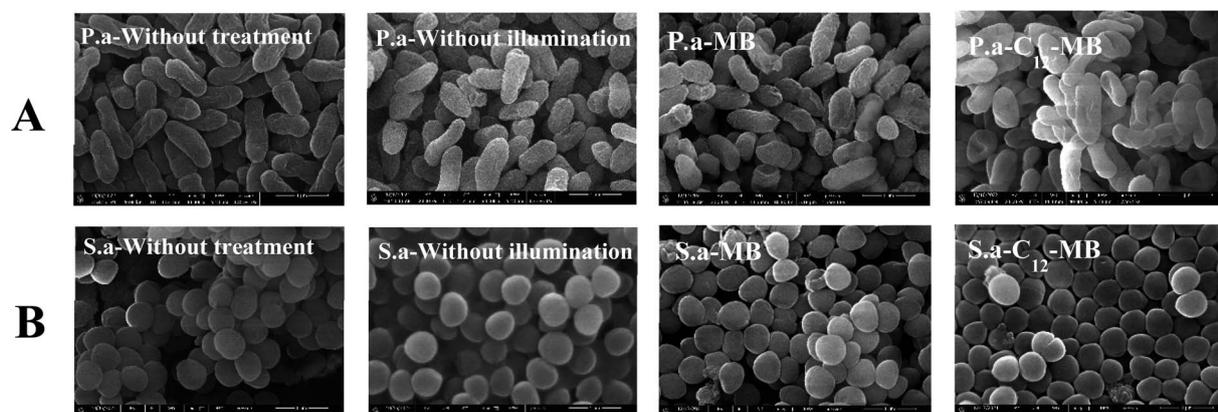
Fig. 5 Bacterial morphology observation by scanning electronic microscopy after photodynamic treatment by MB and C<sub>12</sub>-MB. Images of *P. aeruginosa* (A) and *S. aureus* (B) treated by APDT of without treatment, without illumination, MB and C<sub>12</sub>-MB.
