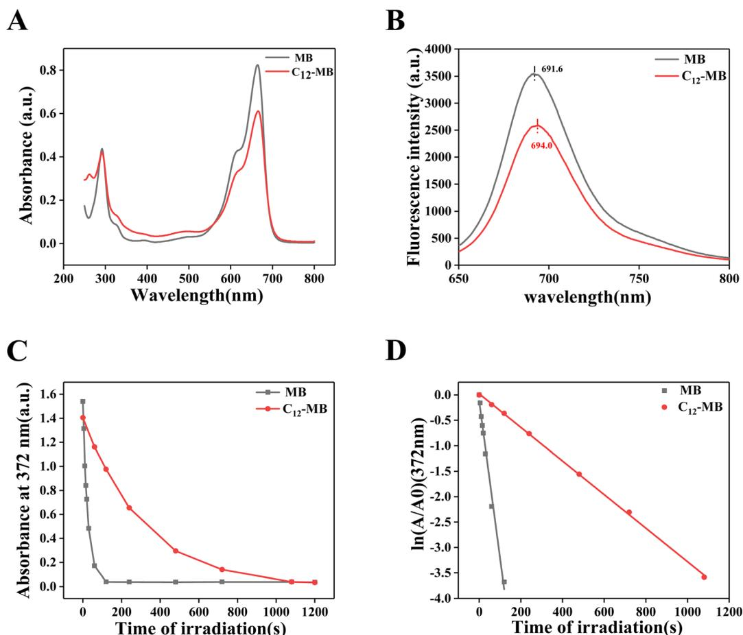
Fig. 3 The photophysical properties of methylene blue and  $C_{12}$ -MB. (A) UV-Vis absorption spectra. Concentration:  $6.25 \mu\text{mol L}^{-1}$ . (B) Intrinsic fluorescence emission spectra. Concentration:  $25 \mu\text{mol L}^{-1}$ . (C) Singlet oxygen productivity (the absorbance decay at 372 nm with different irradiation time) of MB and  $C_{12}$ -MB detected by 9,10-diphenylanthracene oxidation. (D) Singlet oxygen productivity kinetics fitted with a pseudo-first order model.
