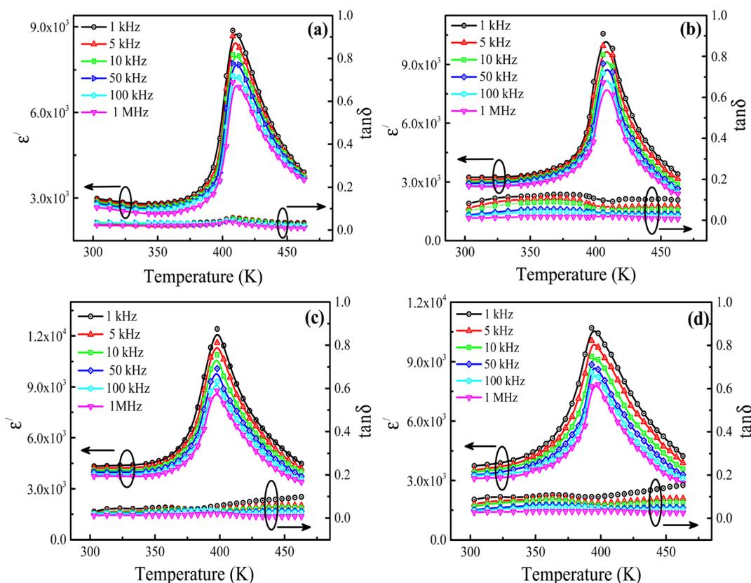
Fig. 3 Temperature-dependent behavior of the real part of dielectric permittivity ( $\epsilon'$ ) and dielectric tangent loss ( $\tan \delta$ ) for the La<sup>3+</sup> doped Ba<sub>1-x</sub>La<sub>x</sub>TiO<sub>3</sub> ceramics (a)  $x = 0.0$ , (b)  $x = 0.0025$ , (c)  $x = 0.005$ , and (d)  $x = 0.0075$  measured at different frequencies (1 kHz to 1 MHz) between the temperature range of 303 K to 463 K.
