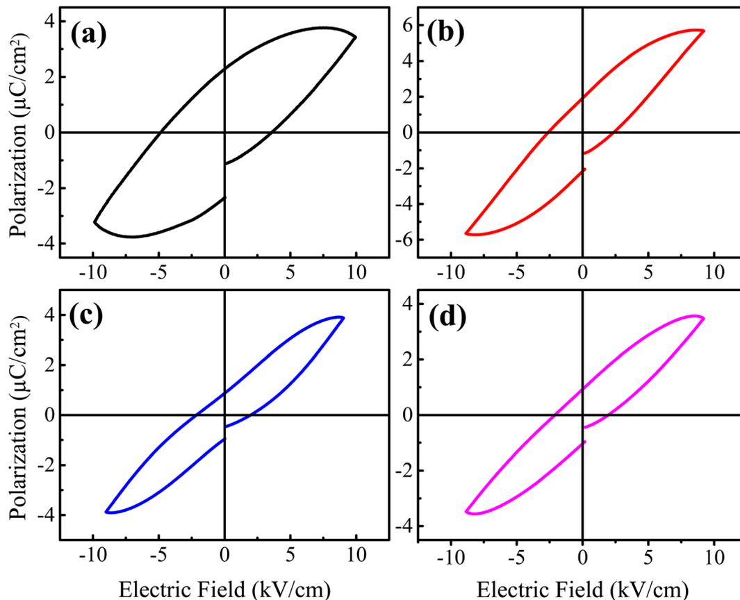
Fig. 8 Ferroelectric hysteresis loops of the prepared  $\text{Ba}_{1-x}\text{La}_x\text{TiO}_3$  ceramics with (a)  $x = 0.0$ , (b)  $x = 0.0025$ , (c)  $x = 0.005$ , and (d)  $x = 0.0075$  measured at room temperature.
