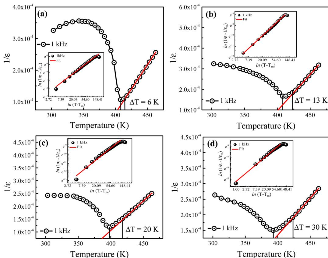
Fig. 4 Temperature dependence of the inverse of dielectric permittivity ( $\epsilon'$ ) for the La<sup>3+</sup> doped Ba<sub>1-x</sub>La<sub>x</sub>TiO<sub>3</sub> ceramics with (a)  $x = 0.0$ , (b)  $x = 0.0025$ , (c)  $x = 0.005$ , and (d)  $x = 0.0075$  measured at a representative frequency of 1 kHz. Insets of (a–d) display the graphs of  $\ln(1/\epsilon_r - 1/\epsilon_m)$  versus  $\ln(T - T_m)$  for the prepared samples.
