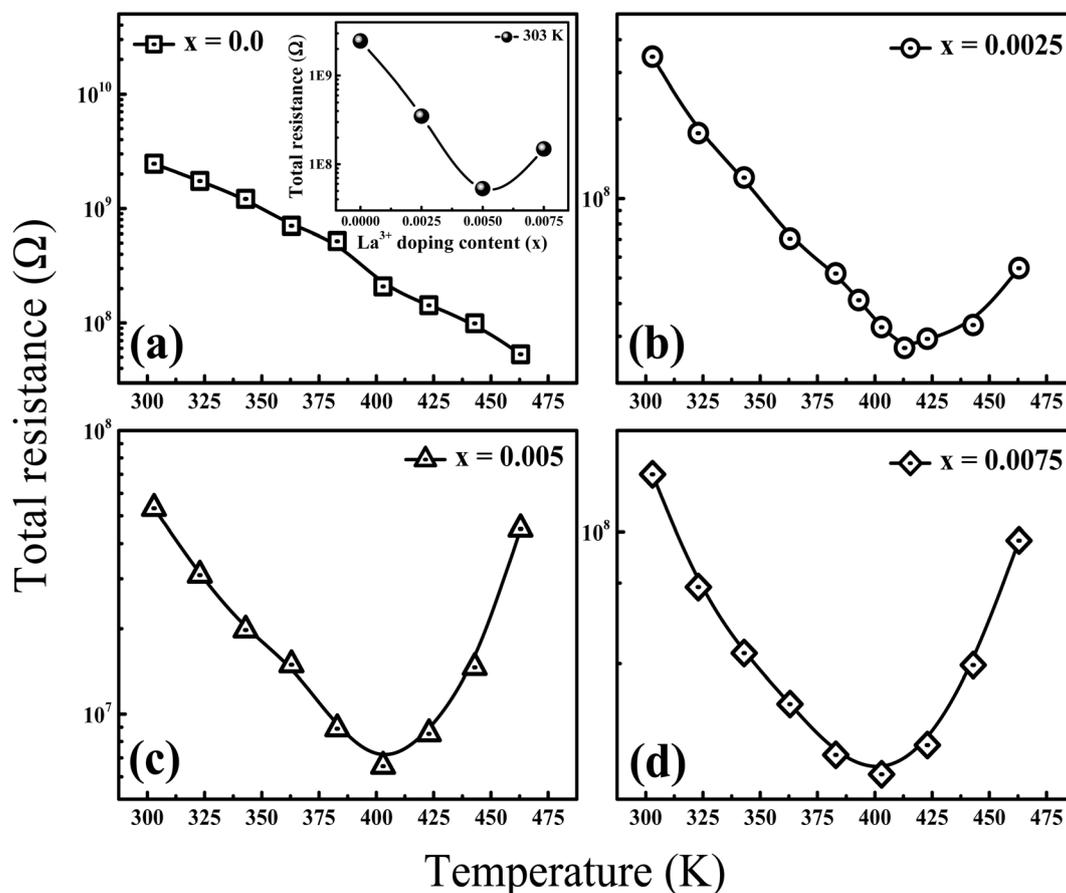
Fig. 6 Temperature dependence of the total resistance ( $R_T$ ) in the prepared  $\text{Ba}_{1-x}\text{La}_x\text{TiO}_3$  ceramics with (a)  $x = 0.0$ , (b)  $x = 0.0025$ , (c)  $x = 0.005$ , and (d)  $x = 0.0075$ . Inset of (a) shows the variation in the magnitude of  $R_T$  with increasing  $\text{La}^{3+}$  doping content ( $x$ ) at room temperature.
