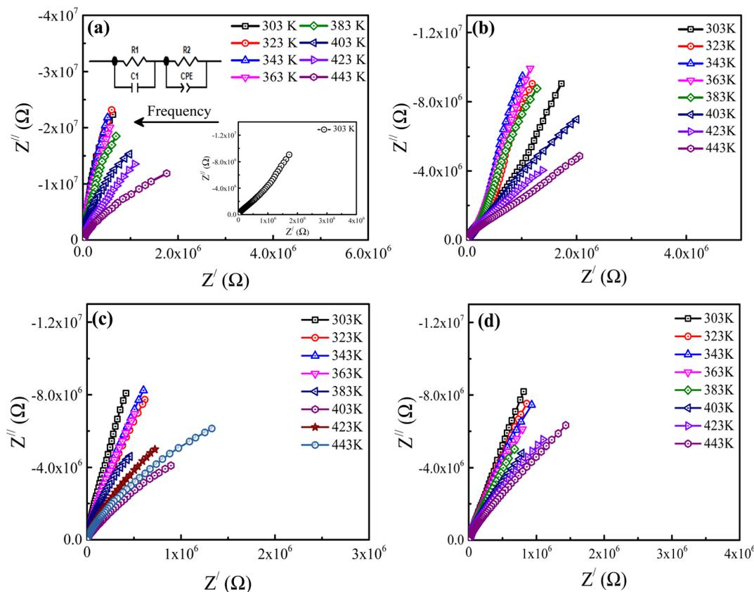
Fig. 5 Complex impedance plane plots ( $Z'$  vs.  $Z''$ ) of  $\text{Ba}_{1-x}\text{La}_x\text{TiO}_3$  ceramics with (a)  $x = 0.0$ , (b)  $x = 0.0025$ , (c)  $x = 0.005$ , and (d)  $x = 0.0075$  measured at various temperatures. Insets of (a) show the enlarged Insets of (a) show the impedance plane plot measured at 303 K and the equivalent circuit model. Here, the arrow shows the direction of the applied frequency.
