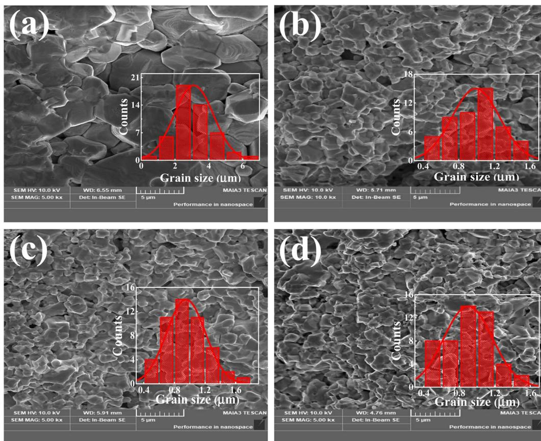
**Fig. 2** SEM micrographs of  $\text{La}^{3+}$  doped  $\text{Ba}_{1-x}\text{La}_x\text{TiO}_3$  ceramics with (a)  $x = 0.0$ , (b)  $x = 0.0025$ , (c)  $x = 0.005$ , and (d)  $x = 0.0075$ . Insets of (a–d) show the grain size distribution.
