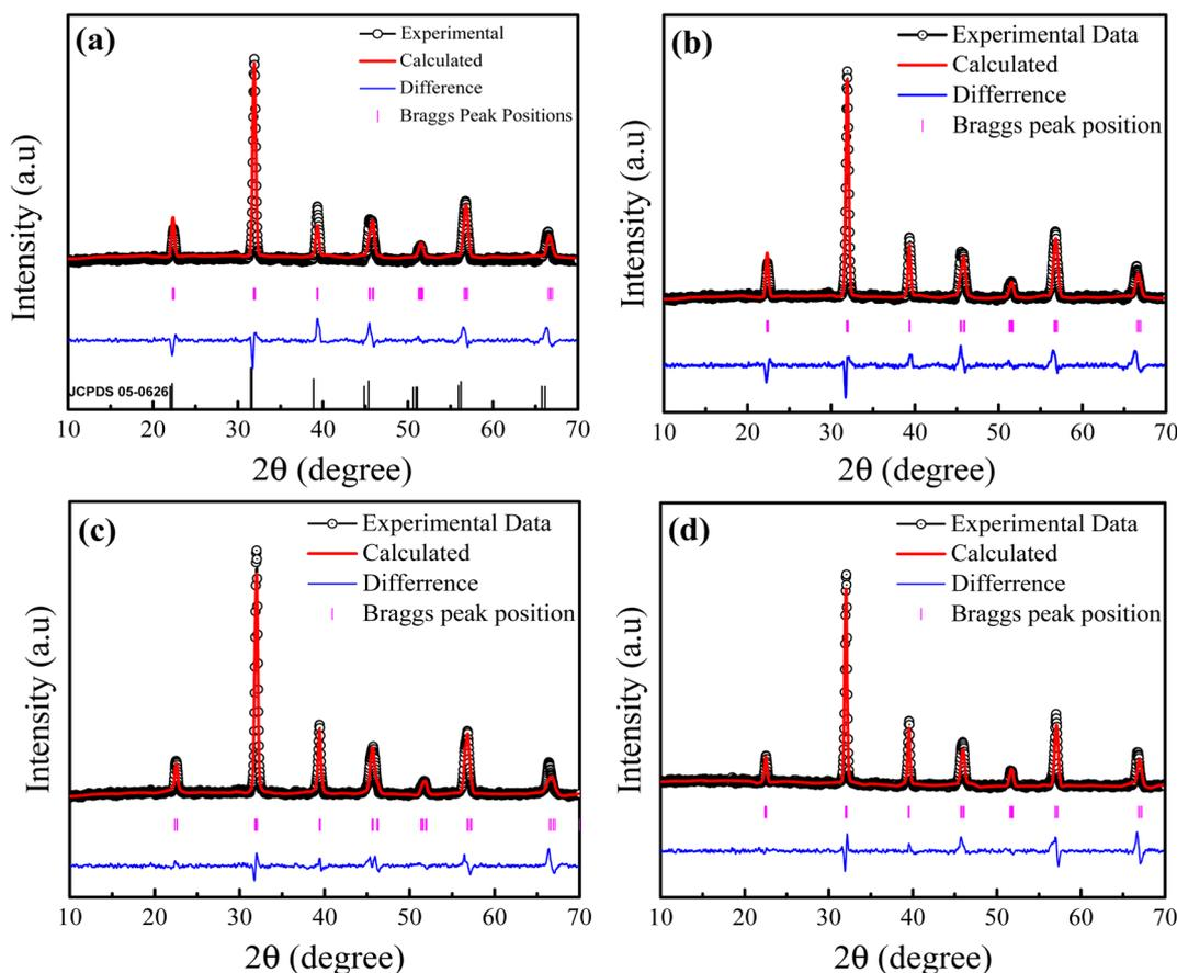
Fig. 1 Rietveld refinement of the XRD data of  $\text{La}^{3+}$  doped  $\text{Ba}_{1-x}\text{La}_x\text{TiO}_3$  ceramics with (a)  $x = 0.0$ , (b)  $x = 0.0025$ , (c)  $x = 0.005$ , and (d)  $x = 0.0075$ . Here, the experimental data are depicted by the black circle, the estimated intensities by the red line, the difference between both intensities by the blue baseline, and the allowed Bragg's position by the magenta vertical lines.
