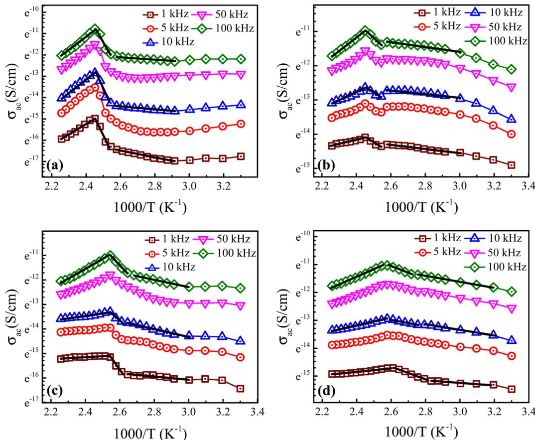
Fig. 7 Temperature-dependent ac conductivity ( $\sigma_{ac}$ ) behavior of the prepared  $\text{Ba}_{1-x}\text{La}_x\text{TiO}_3$  ceramics with (a)  $x = 0.0$ , (b)  $x = 0.0025$ , (c)  $x = 0.005$ , and (d)  $x = 0.0075$  at different frequencies (1 kHz–100 kHz). Solid lines show the fit to the experimental data using eqn (6) at different frequency regions.
