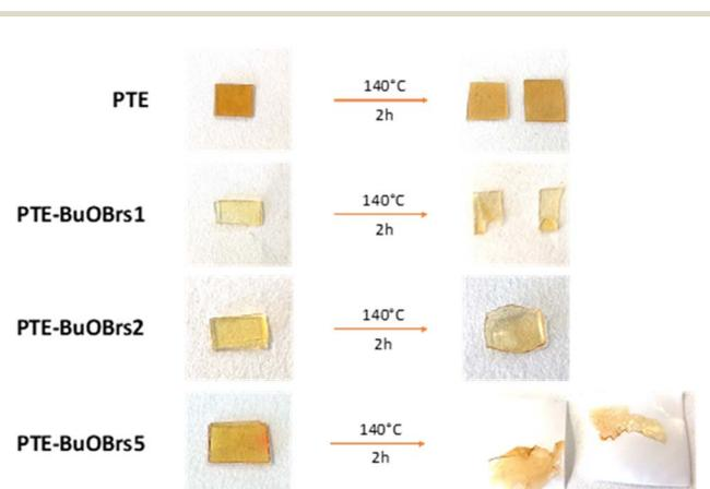
Fig. 2 Healing behavior of PTE-BuOBr5 samples and PTE control sample at 140 °C during 2 h.
