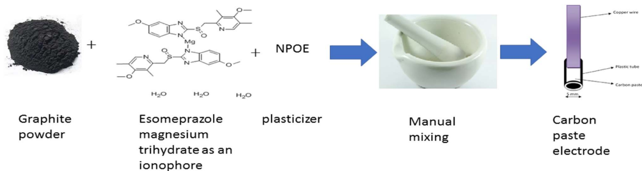
Fig. 2 Diagram for the fabrication process of esomeprazole magnesium sensor.
