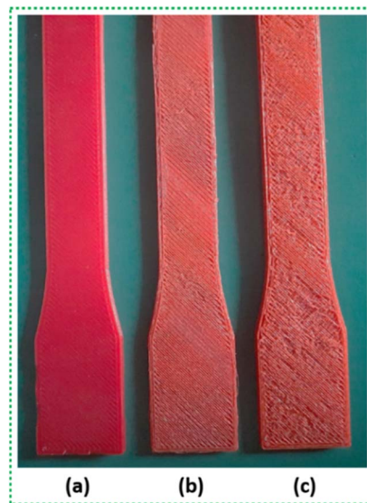
Fig. 8 Sample PLA surface for (a) PLA-0, (b) PLA-30 and (c) PLA-45.
