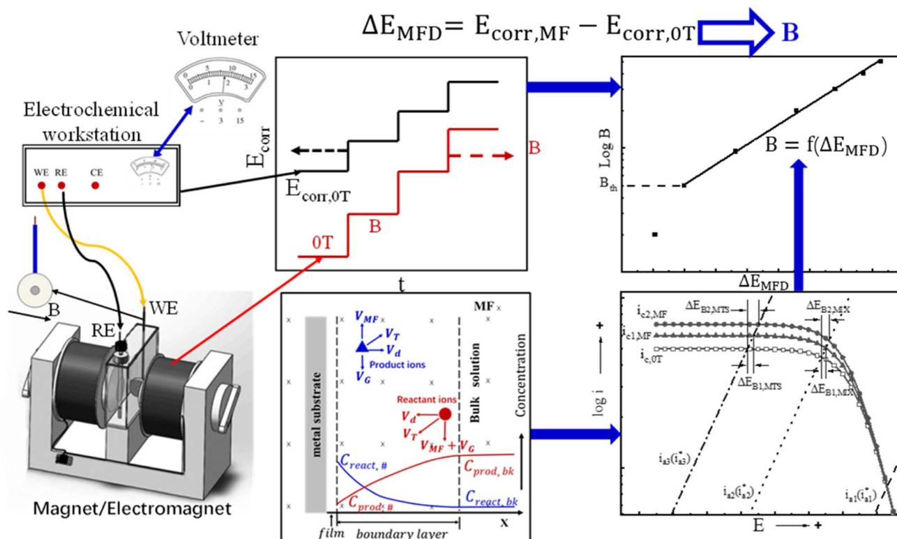
Fig. 1 The roadmap for measuring the MFD.
