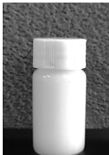
Fig. 2 Optical photos of AGE-CA self-emulsifying solution after six months at room temperature.
