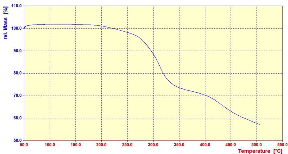
Fig. 5 TGA curves of CS-TDI-Me-TDI-HNSO 3 H organocatalyst (1).
