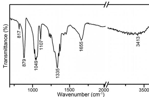
Fig. 3 FTIR spectrum of the 6535BBN/AgBr composite.
