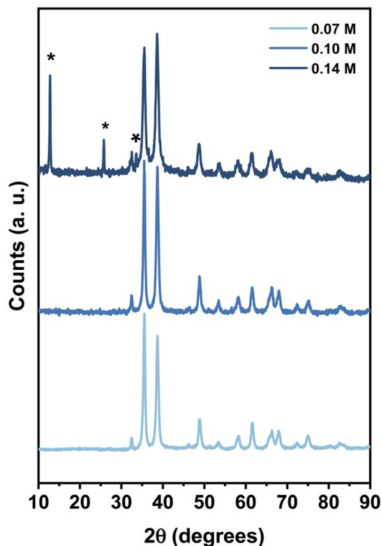
Fig. 1 XRD pattern of the CuO samples prepared with different concentrations of Cu<sup>2+</sup>.
