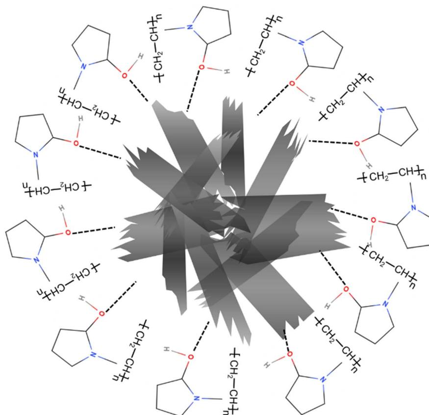
Fig. 5 Schematic diagram of the interaction of PVP chains with CuO nanosheets through H-bonding.
