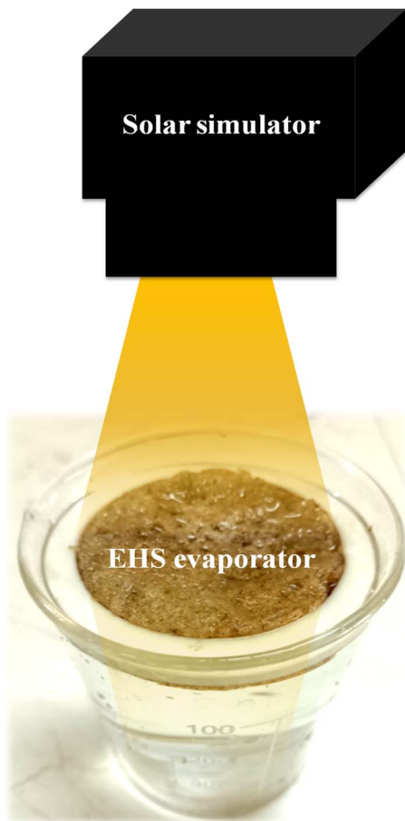
Fig. 3 Solar steam generation experimental setup.
