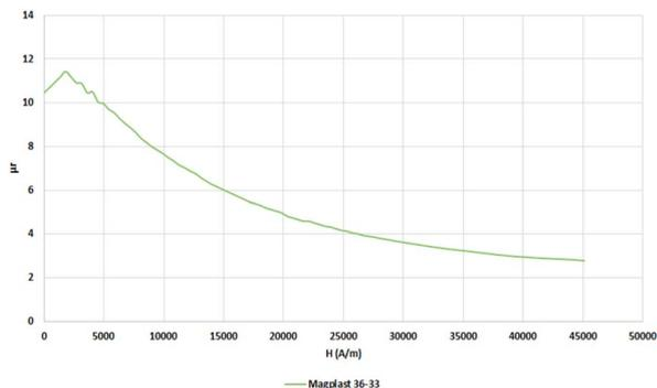
Fig. 5 Permeability vs. magnetic field  $H$  ( $\text{A m}^{-1}$ ) of MagPlast 36-33.
