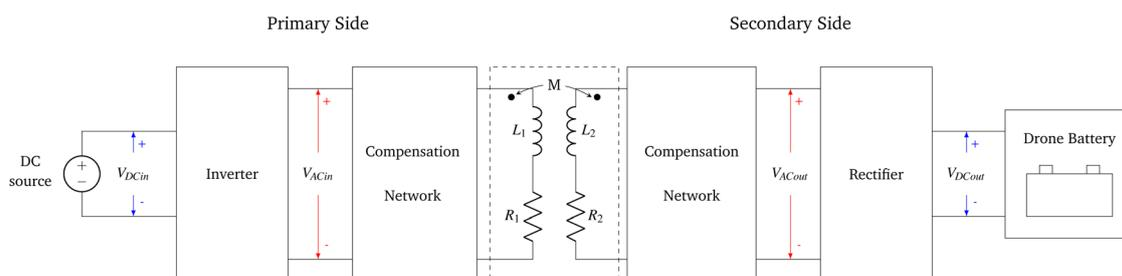
Fig. 1 Generic scheme of the WPT drone charger.
