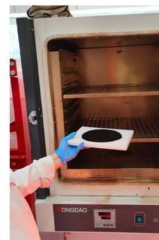
(b) Mould placed in the oven.
