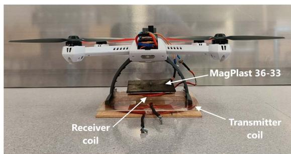
Fig. 12 Drone assembly with MagPlast 36-33.
