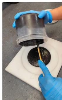
(a) Mixture added into the mould.
