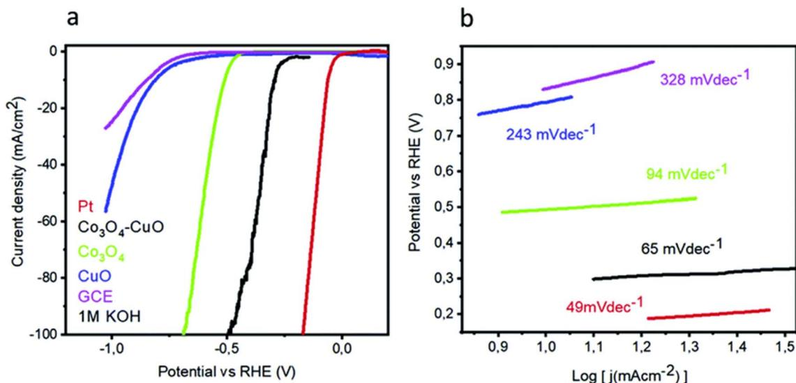
Fig. 6 (a) LSV and (b)  $\text{Co}_3\text{O}_4$ ,  $\text{CuO}$ , and  $\text{Co}_3\text{O}_4$ - $\text{CuO}$  nano-based composites Tafel slopes (reproduced with permission from Elsevier, copyright 2019).<sup>153</sup>
