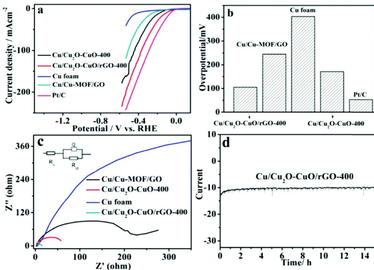
Fig. 5 (a) LSV, (b) value of overpotential at the assigned current density, (c) electrochemical impedance study, and (d) chromatography results obtained for 14 hours trials (reproduced with permission from RSC, copyright 2018).<sup>152</sup>
