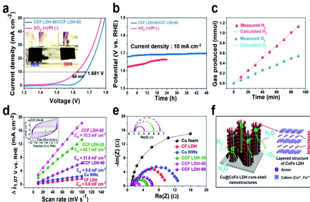
Fig. 7 (a) LSV, (b) GSTAT analysis, (c) faradaic efficiency, (d) ECSA, (e) Nyquist plot, and (f) the structure of Cu@CoFeLDH over Cu foam (reproduced with permission from Elsevier, copyright 2019).<sup>154</sup>
