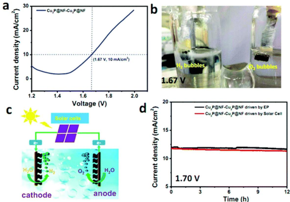
Fig. 16 (a–d) LSV, Cu<sub>3</sub>P catalysts in KOH for two-electrodes, the scheme, and PSTAT analysis for 12 h (reproduced with permission).<sup>172</sup>
