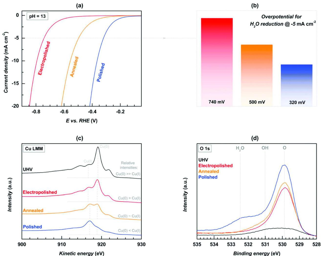
Fig. 4 (a) LSV, (b) value of overpotential at the assigned current density, (c) XPS of Cu-LMM, and (d) spectra of high resolution for O 1s (reproduced with permission from Elsevier, copyright 2019).<sup>151</sup>
