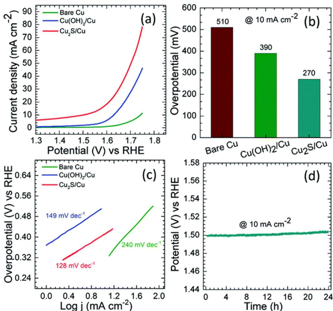
Fig. 10 (a–d) showing LSV, overpotential at  $10 \text{ mA cm}^{-2}$ , Tafel slope, and chronopotentiometry respectively (reproduced with permission from RSC, copyright 2020).<sup>159</sup>
