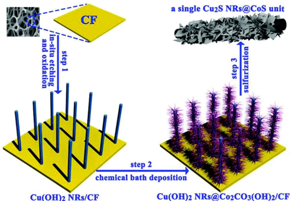
Fig. 12 Process description of CoS-shelled  $\text{Cu}_2\text{S}$  nanorods over Cu foam (reproduced with permission from Elsevier, copyright 2019).<sup>165</sup>
