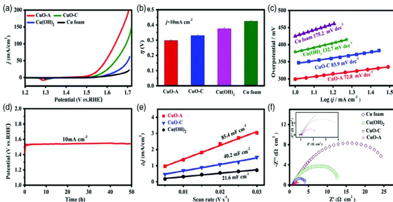
Fig. 13 (a–f) LSV, overpotential at 10 mA cm<sup>-2</sup>, Tafel slope, chronopotentiometry, ECSA, and EIS results of CuO–A, CuO–C, and Cu(OH)<sub>2</sub> (reproduced with permission from ACS publications, copyright 2018).<sup>168</sup>
