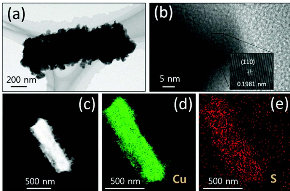
Fig. 9 (a–e)  $\text{Cu}_2\text{S}$  over the Cu based substrate HAADF mapping and HRTEM imaging (reproduced with permission from ACS Publications, copyright 2018).<sup>159</sup>
