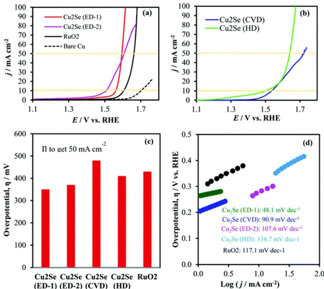
Fig. 14 (a) and (b) LSV, (c) overpotential at 50 mA cm<sup>-2</sup>, and (d) the Tafel slope results of Cu<sub>2</sub>Se catalysts (reproduced with permission from ACS publications, copyright 2018).<sup>168</sup>
