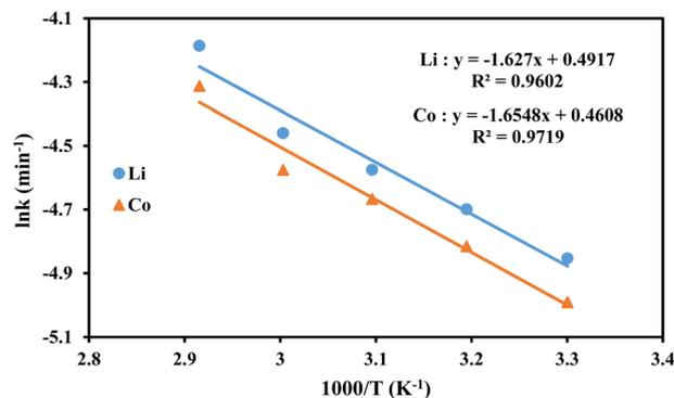
Fig. 10 Arrhenius plot for the leaching of Li and Co.
