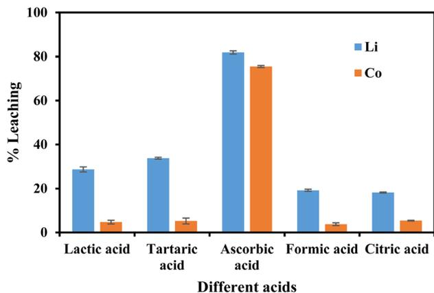
Fig. 2 Effect of different organic acids on the leaching efficiency of Li and Co (acid conc. =  $0.5 \text{ mol L}^{-1}$ , S/L =  $10 \text{ g L}^{-1}$ , temperature =  $30 \text{ }^\circ\text{C}$ , leaching time = 60 min, particle size =  $-25 \mu\text{m}$ ).
