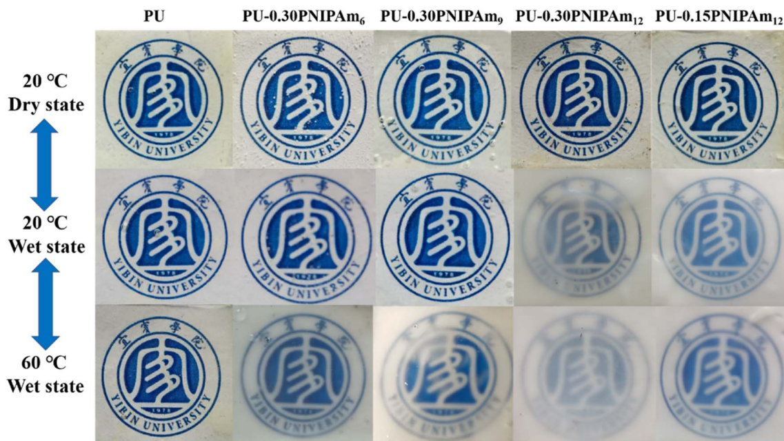
Fig. 9 The digital photographs of all samples at 20 °C (dry state, top), 20 °C (wet state, middle) and 60 °C (wet state, bottom).
