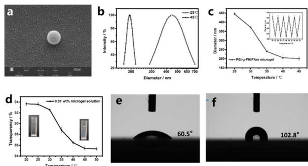
**Fig. 3** (a) SEM of the PEI-*g*-PNIPAm microgel. (b) The PEI-*g*-PNIPAm microgel's size and its dispersion in 25 °C and 45 °C. (c) The PEI-*g*-PNIPAm microgel's size at different temperature (insert: the size's cycle ability between 25 °C and 45 °C). (d) The microgel's transparency at different temperature. (e) The microgel film's contact angle at 25 °C. (f) The microgel film's contact angle at 45 °C.
