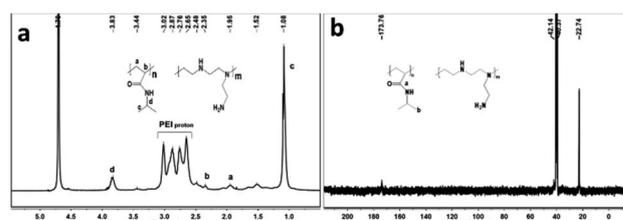
Fig. 2 (a) The <sup>1</sup>H-NMR in D<sub>2</sub>O and (b) the <sup>13</sup>C-NMR in deuterated DMSO of the PEI-*g*-PNIPAM microgel.
