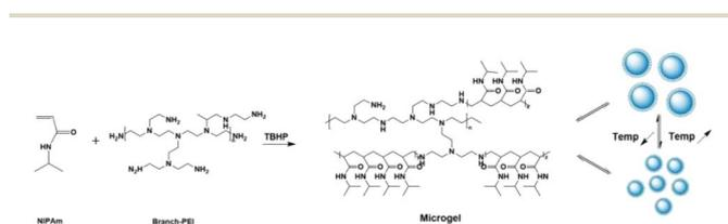
Fig. 1 The process to prepare the microgel.
